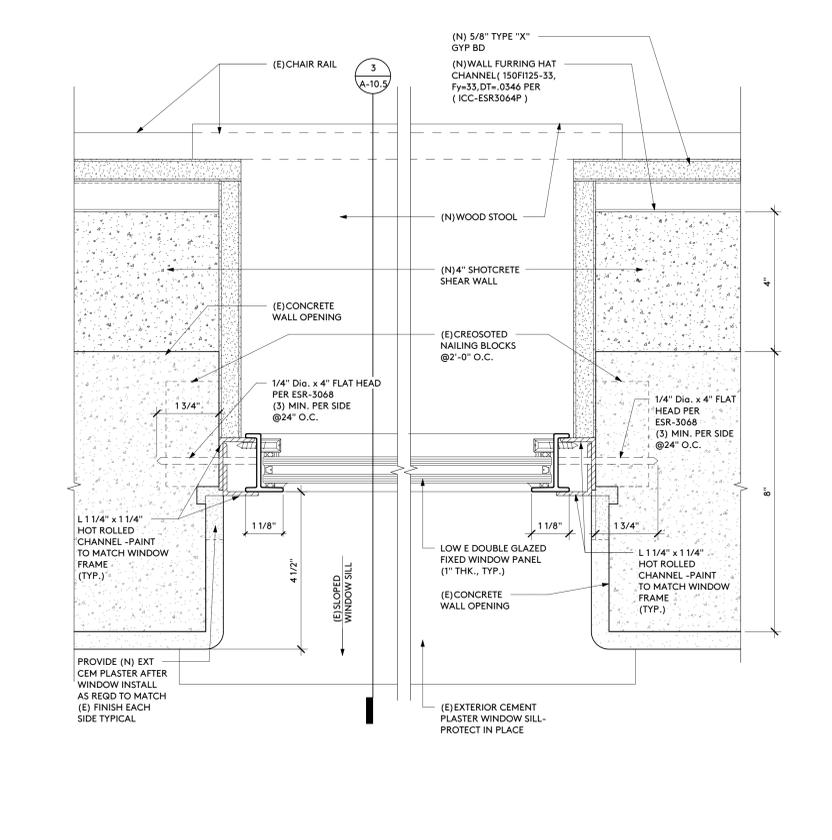
**STEEL WINDOW JAMB @ SHOTCRETE SHEAR WALL** 4
