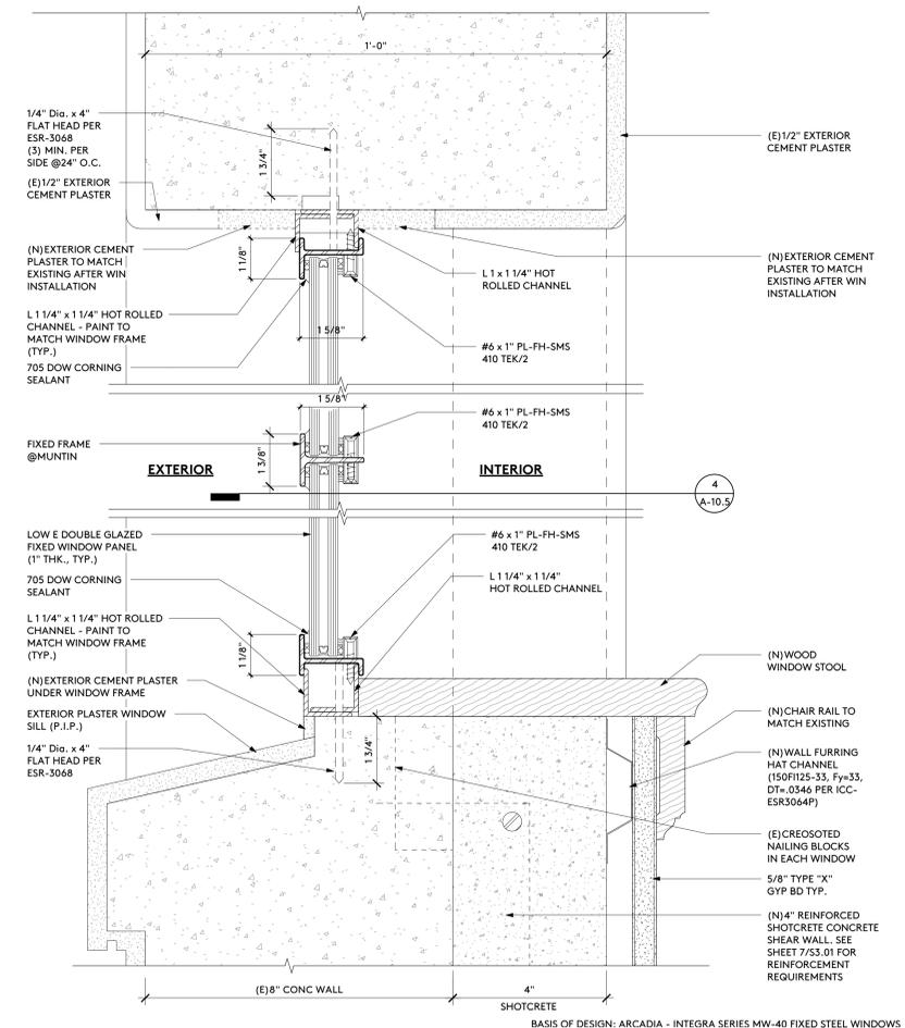
**STEEL WINDOW @ JAMB & SILL W/ SHOTCRETE SHEAR WALL** 3
