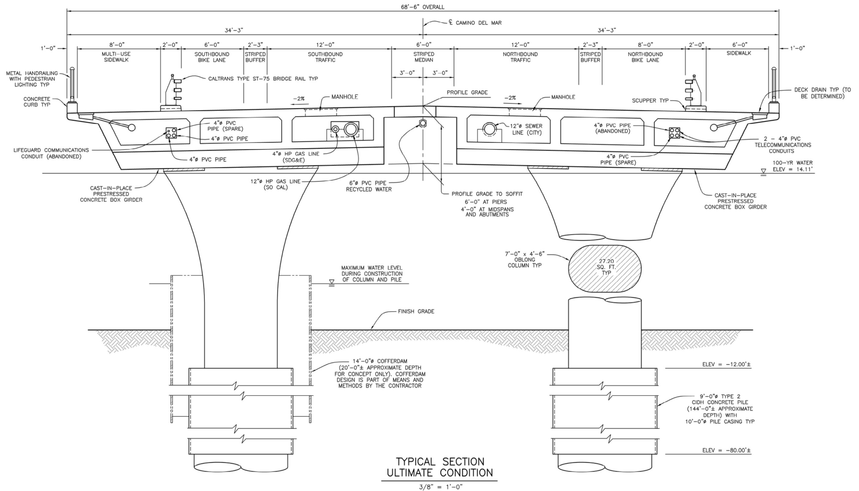
ALTERNATIVE 2.1: 6-SPAN VARIABLE DEPTH CAST-IN-PLACE PRESTRESSED CONCRETE BOX GIRDER BRIDGE WITH TWO COLUMNS PER PIER (BASELINE)
