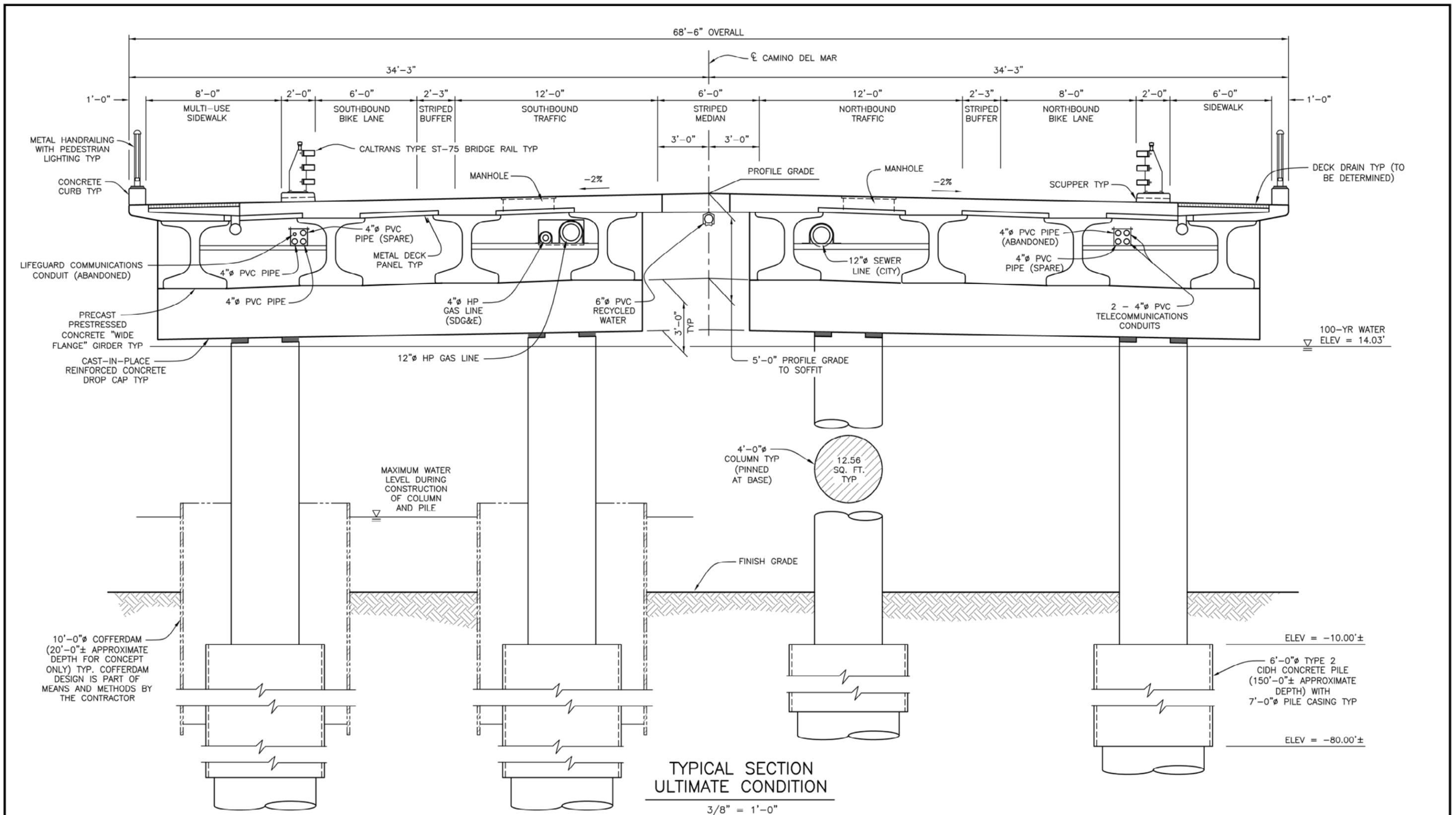
ALTERNATIVE 9.2: 6-SPAN PRECAST PRESTRESSED CONCRETE WIDE-FLANGE GIRDER BRIDGE WITH FOUR COLUMNS PER PIER
