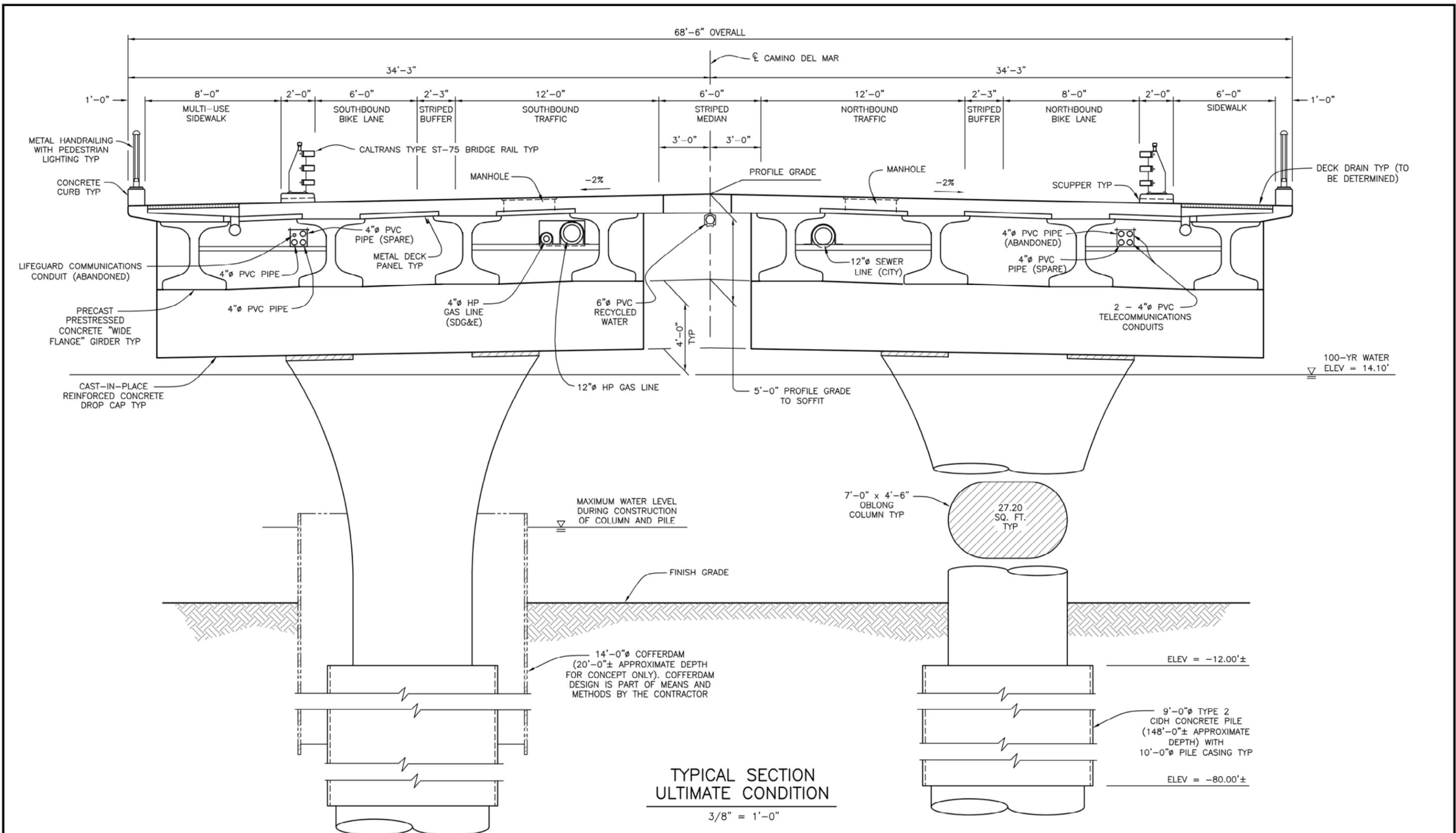
**ALTERNATIVE 9.1: 6-SPAN PRECAST PRESTRESSED CONCRETE WIDE-FLANGE GIRDER BRIDGE WITH TWO COLUMNS PER PIER**
