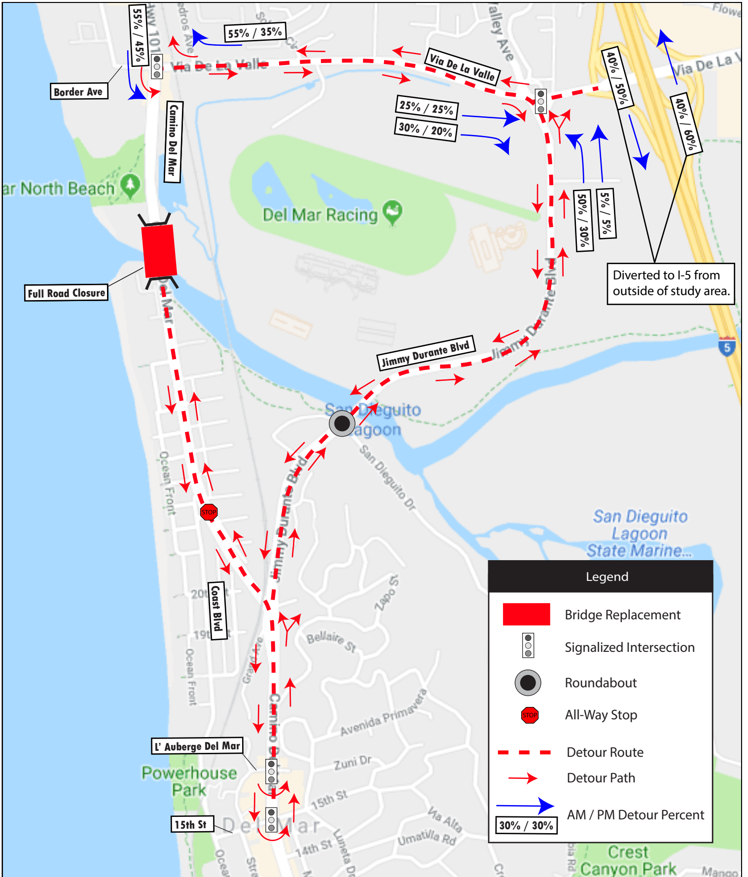
Figure 5-7 Potential Traffic Diversion for Full Closure Construction Scenario
