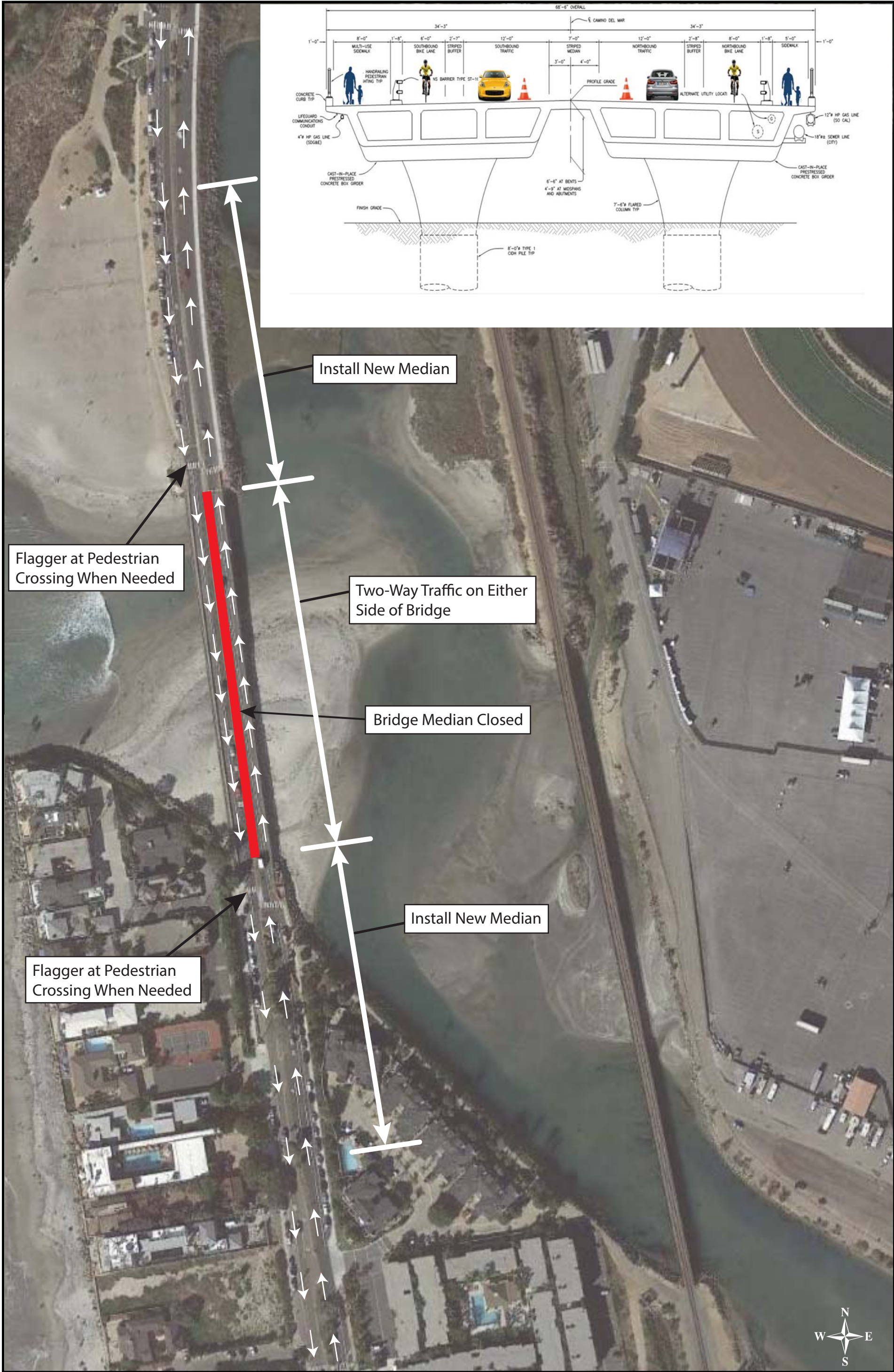
Figure 5-3 Bridge Median Construction Stage Traffic Control Plan Concept
