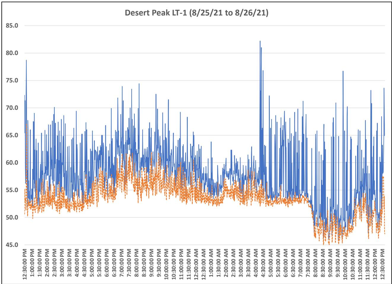
**Figure 4.** Plot of  $L_{eq}$  (solid blue line) and  $L_{90}$  (dashed orange line) values per successive one-minute intervals
