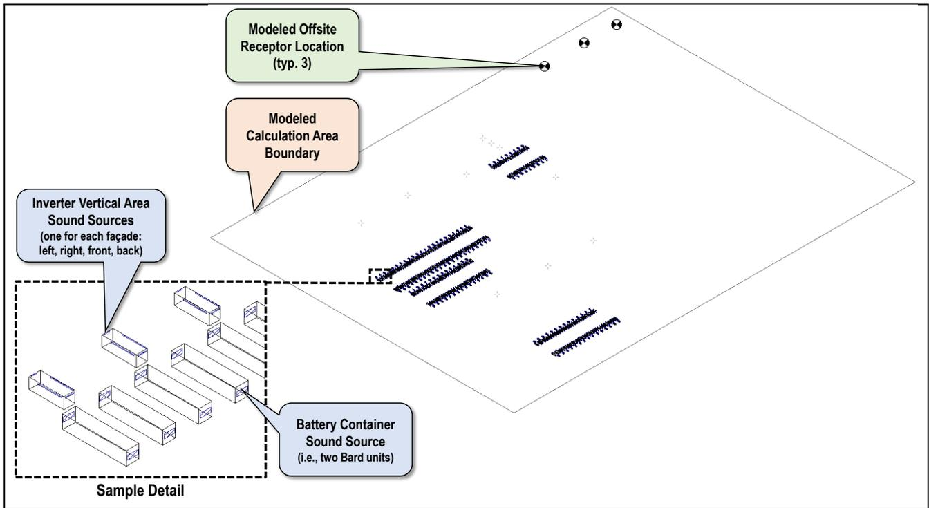
**Figure 2.** Isometric view, looking northwest, of Phase 2 site CadnaA prediction model and enlarged sample features
