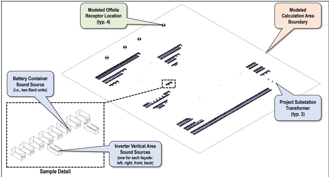
**Figure 1.** Isometric view, looking northwest, of Phase 1 site CadnaA prediction model and enlarged sample features
