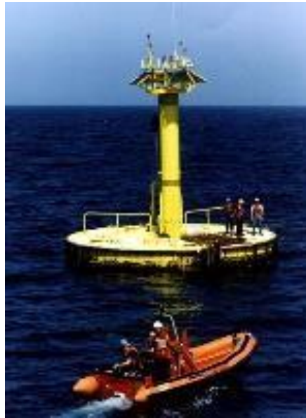
Figure 2-4: 10-Meter Discus-Shaped Hull Buoy
