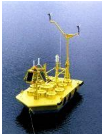
Figure 2-5: 6-Meter Boat-Shaped Hull Buoy
