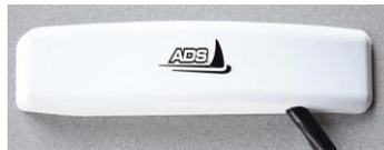
The **ADS FlowShark Triton** monitor was selected for this project. This flow monitor is an area velocity flow monitor that uses both the Continuity and Manning's equations to measure flow.
