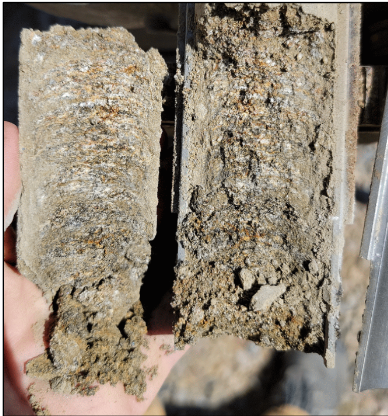
Figure 4-3. Granitic Rock in Boring B-4
