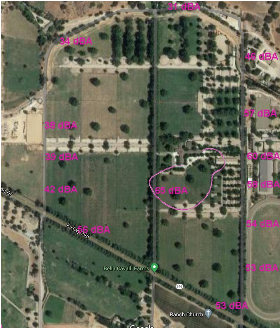
Figure 2: Predicted, property line sound levels from Site 1, southeast of the existing barn.
