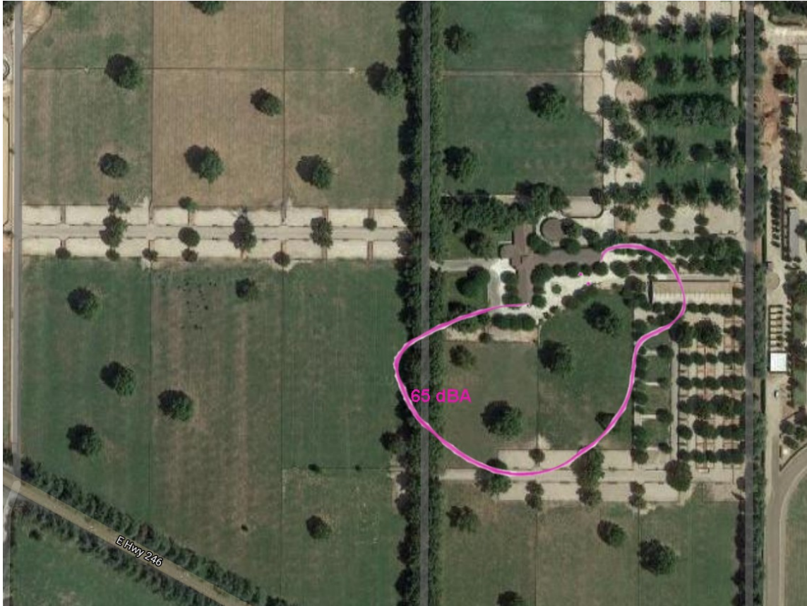
Figure 1: Predicted, 65 dBA sound level contour in the area around Site 1, southeast of the existing barn.
