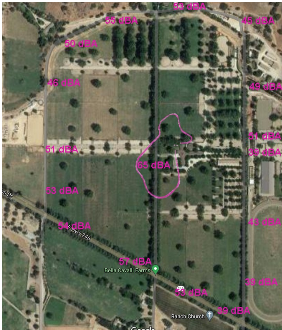
Figure 4: Predicted, property line sound levels from Site 2, northwest of the existing barn.
