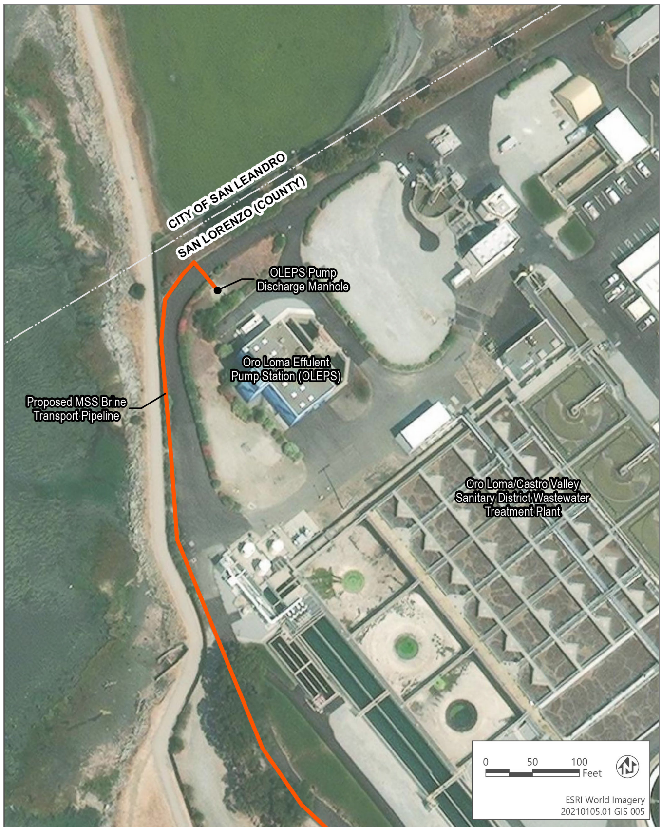
Figure 2-9 MSS Brine Transport Pipeline Connection to the EBDCA Combined Effluent Conveyance System
