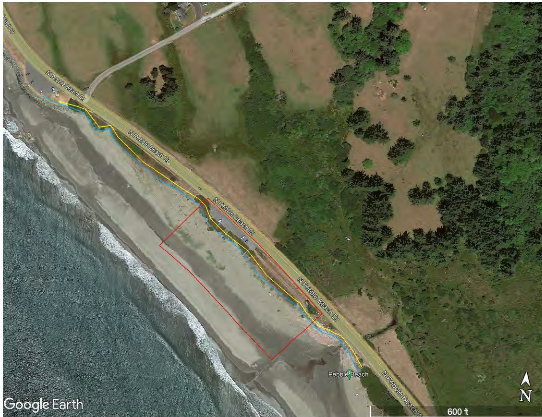
Figure 7: Graphic of estimated bluff retreat in 50 years. Red box is project area, blue line is existing bluff edge, yellow line is projected 50-year retreat extent.
