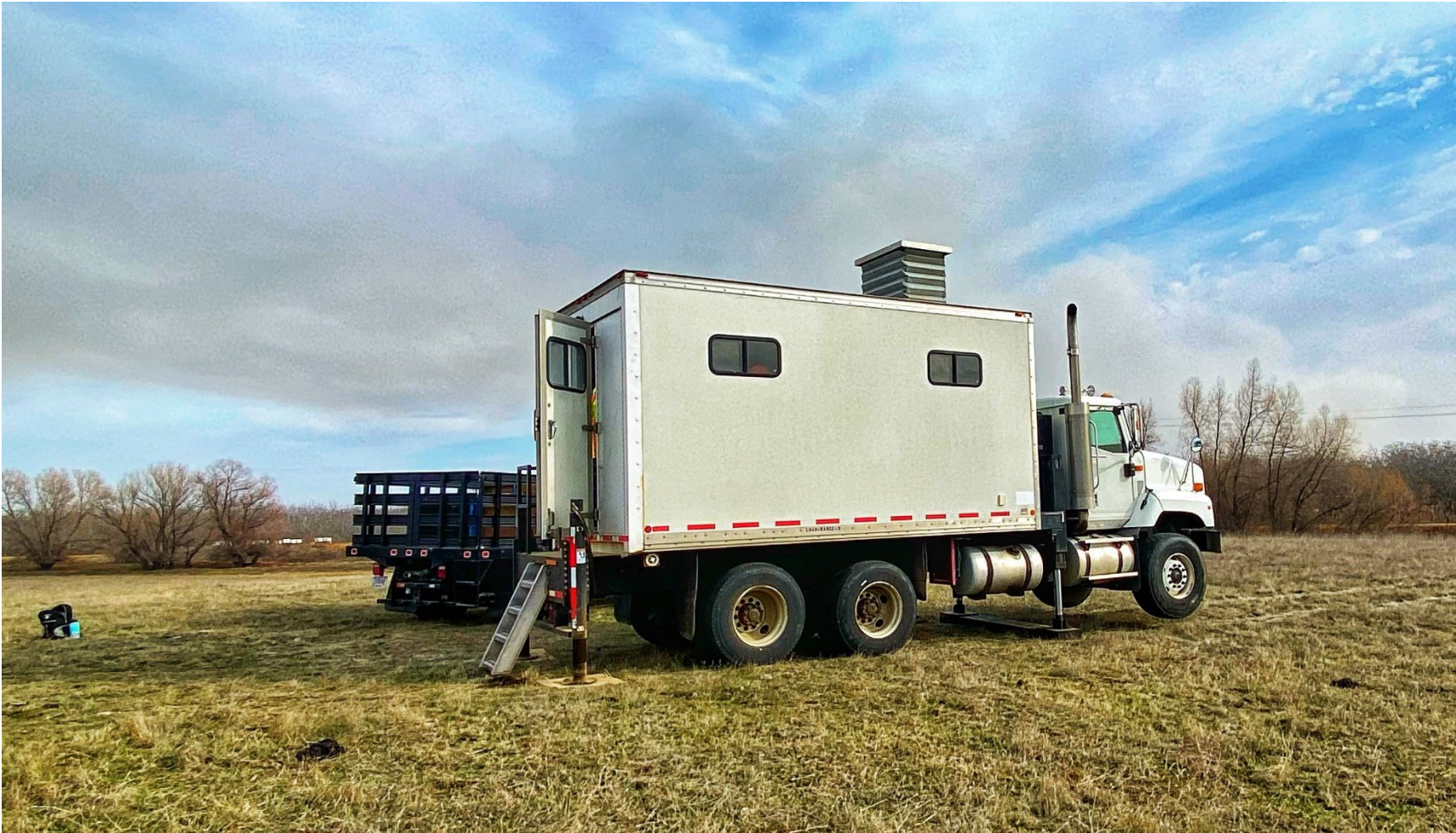
Photo 3 – Representative photo of CPT in grass field
