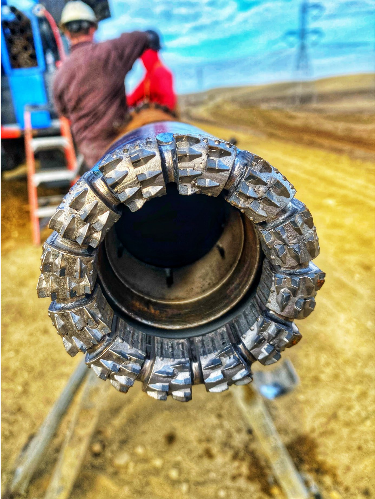
Photo 5 – Representative photo of boring equipment for rock substrate.
