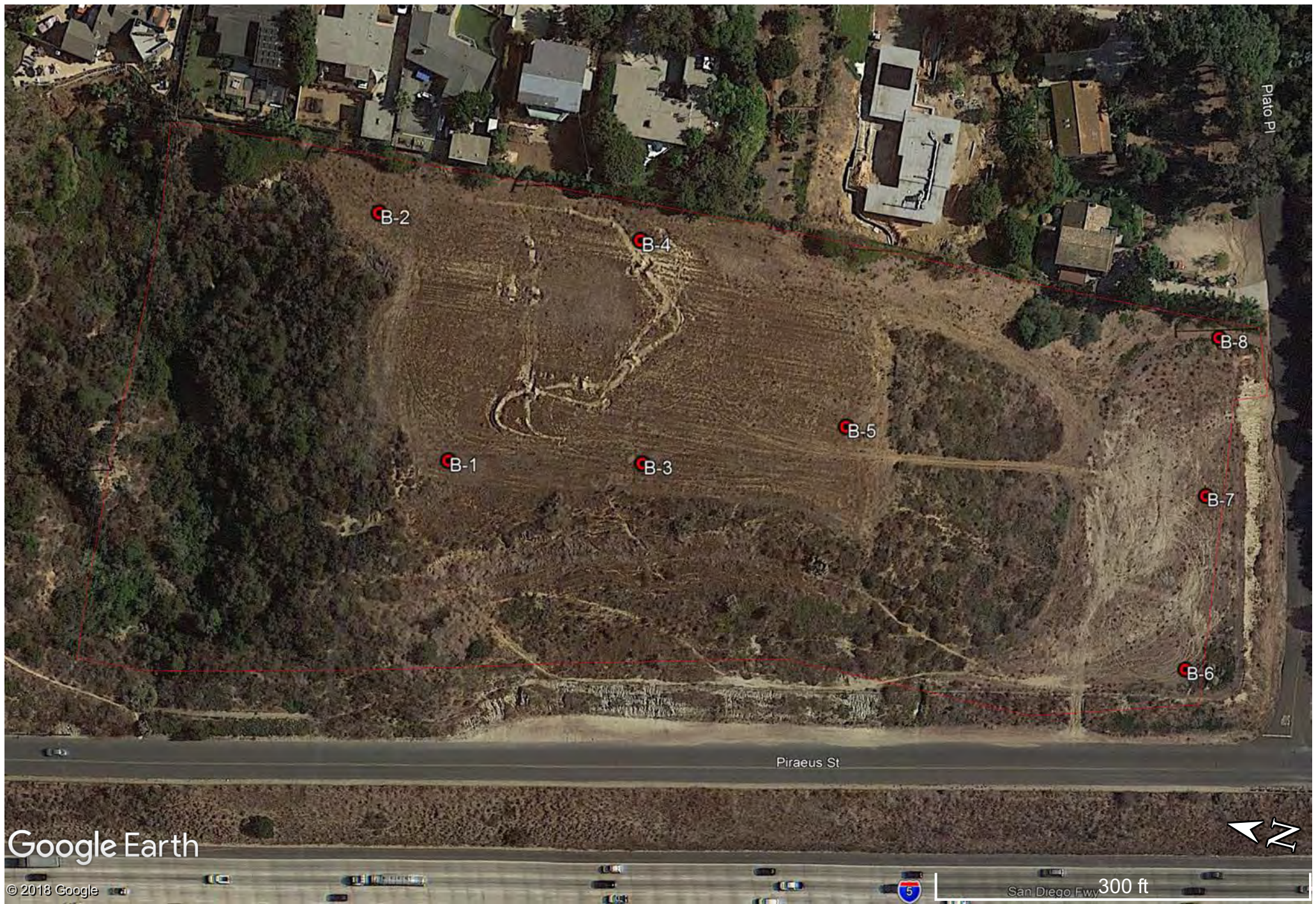
Figure 2 - Boring Location Plan
