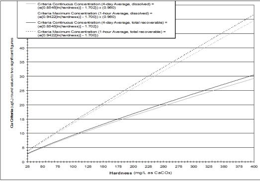
Figure 2. Copper Criteria vs. Hardness Graph
