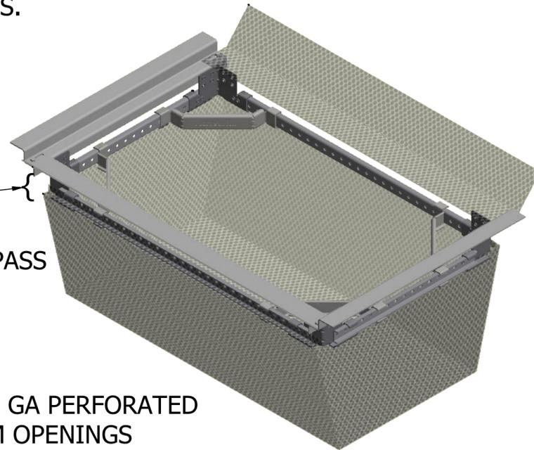
TRASH CAPTURE BASKET: 14 GA PERFORATED STAINLESS STEEL WITH 5MM OPENINGS
