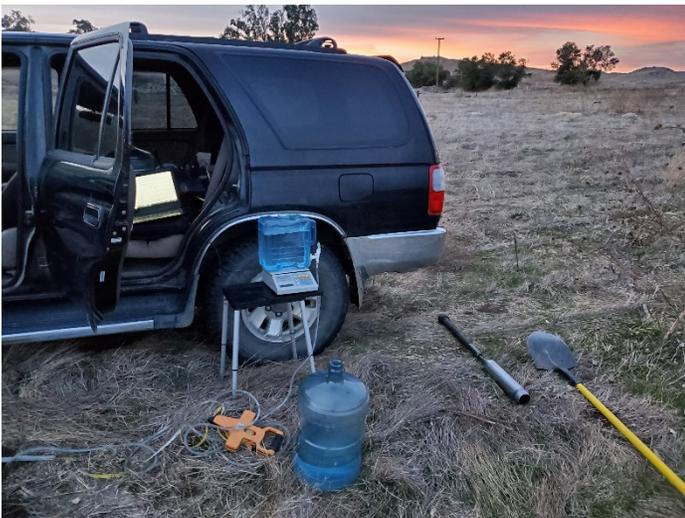
The infiltration tests were conducted in a 3 inch diameter test hole, at depths of 2 to 3 feet deep. The approximate locations of the infiltration test holes are indicated on the attached Infiltration Location Map, Plate 1. Infiltration test holes were located by property boundary measurement on the site plan and/or by using geographic features. The test holes were filled with water and allowed to stand for an extended period of time.
