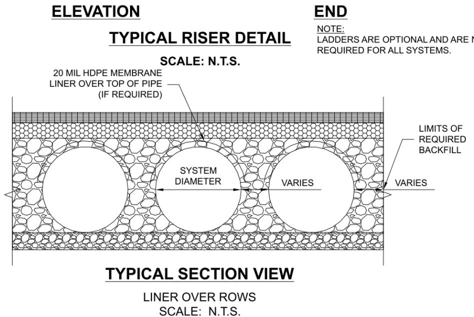
NOTE: IF SALTING AGENTS FOR SNOW AND ICE REMOVAL ARE USED ON OR NEAR THE PROJECT, AN HDPE MEMBRANE LINER IS RECOMMENDED WITH THE SYSTEM. THE IMPERMEABLE LINER IS INTENDED TO HELP PROTECT THE SYSTEM FROM THE POTENTIAL ADVERSE EFFECTS THAT MAY RESULT FROM A CHANGE IN THE SURROUNDING ENVIRONMENT OVER A PERIOD OF TIME. PLEASE REFER TO THE CORRUGATED METAL PIPE DETENTION DESIGN GUIDE FOR ADDITIONAL INFORMATION.
