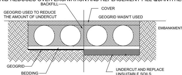
GRADE THE FOUNDATION SUBGRADE TO A UNIFORM OR SLIGHTLY SLOPING GRADE. IF THE SUBGRADE IS CLAY OR RELATIVELY NON-POROUS AND THE CONSTRUCTION SEQUENCE WILL LAST FOR AN EXTENDED PERIOD OF TIME, IT IS BEST TO SLOPE THE GRADE TO ONE END OF THE SYSTEM. THIS WILL ALLOW EXCESS WATER TO DRAIN QUICKLY, PREVENTING SATURATION OF THE SUBGRADE.
