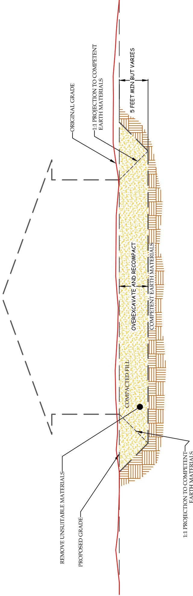
NOTE: REMOVAL BOTTOMS SHOULD BE GRADED WITH A MINIMUM 2% FALL TOWARDS STREET OR OTHER SUITABLE AREA (AS DETERMINED BY THE GEOTECHNICAL CONSULTANT) TO AVOID PONDING BELOW THE BUILDING
