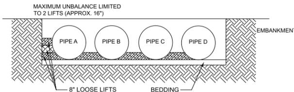
IF AASHTO T99 PROCEDURES ARE DETERMINED INFEASIBLE BY THE GEOTECHNICAL ENGINEER OF RECORD, COMPACTION IS CONSIDERED ADEQUATE WHEN NO FURTHER YIELDING OF THE MATERIAL IS OBSERVED UNDER THE COMPACTOR, OR UNDER FOOT, AND THE GEOTECHNICAL ENGINEER OF RECORD (OR REPRESENTATIVE THEREOF) IS SATISFIED WITH THE LEVEL OF COMPACTION.
