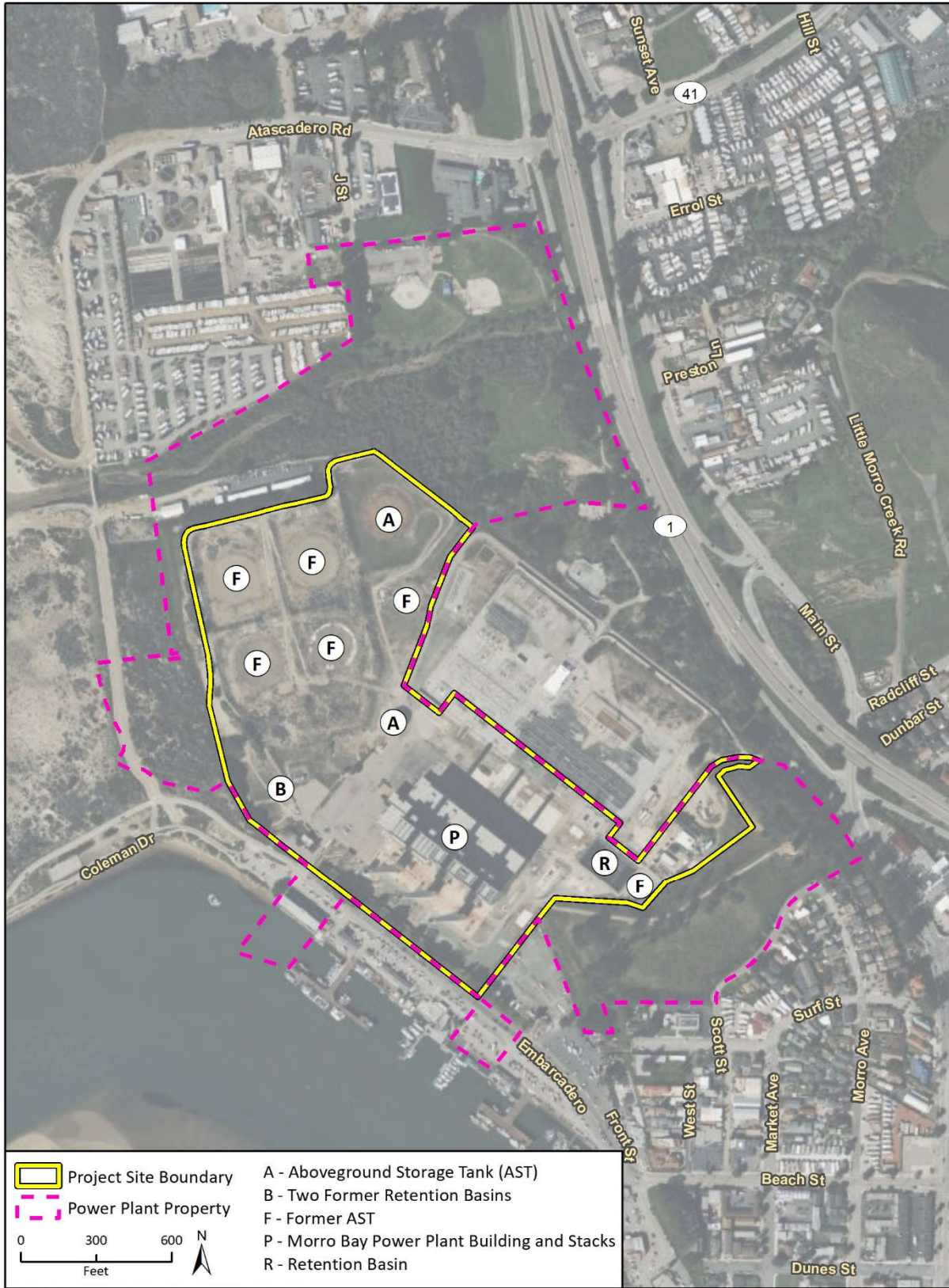
Figure 7 Areas of Hazardous Materials Concern
