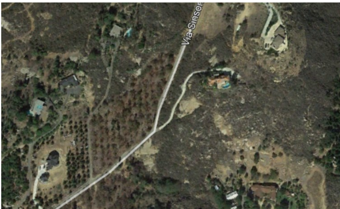
Figure 6. Example of “lower density” development. Homes are interspersed amongst wildland fuels, are of varying ages, and include varying levels of fuel modification zone setbacks. Homes are exposed on most or all sides by flammable vegetation and properties rely solely on owners for maintenance, are often far distances from the nearest fire station, and have minimal buffer from on-site fire spreading to wildlands.
