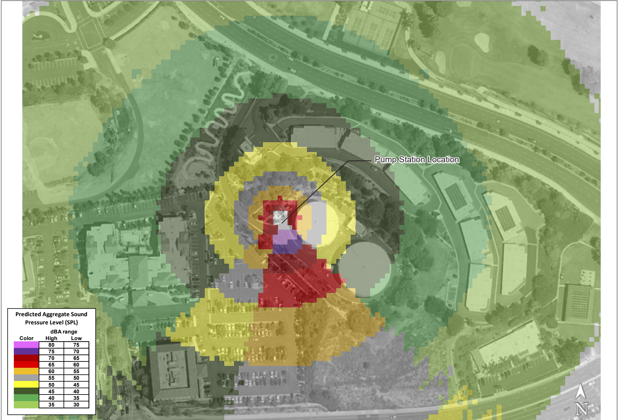
FIGURE 9 Predicted Pump Noise Emission from Station Building El Toro Water District Joint Transmission Main Pump Station Project
