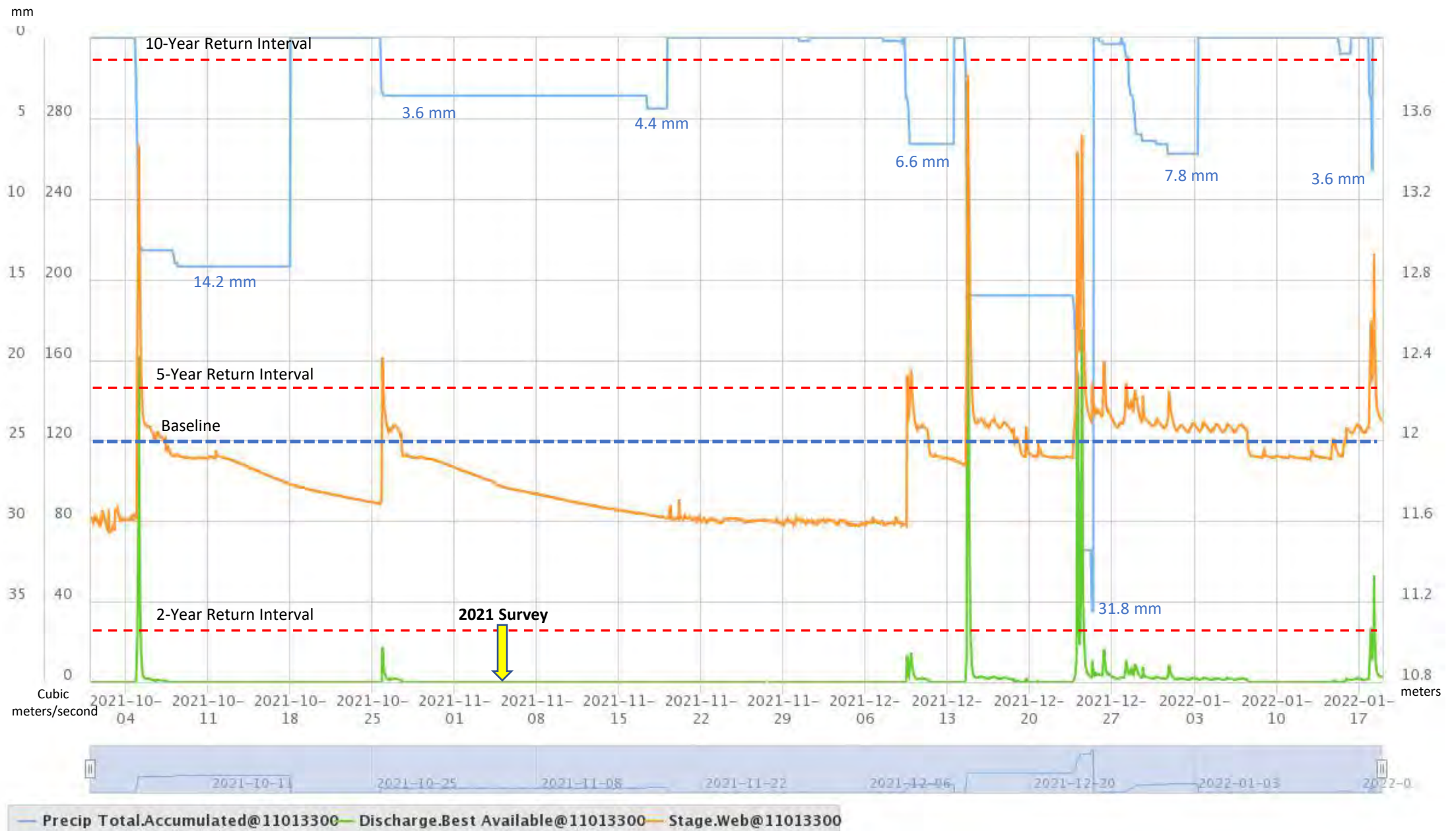
USIBWC gage reported flow discharge, stage height, and accumulated precipitation from October 2021 through January 18, 2022. Prior to the 2021 survey, a less than 2-year discharge event was reported one-week prior, which resulted in overbank flows. Additionally, a 5-year event was reported approximately 1-month prior. Horizontal Lines indicate flood intervals; baseline refers to stage height at approximate floodplain elevation.
