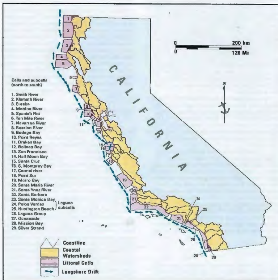
Figure 6: Major littoral cells, coastal watersheds, and conceptual net longshore drift directions for the California coast, modified from Habel and Armstrong (1977) and Hapke et al. (2006).
