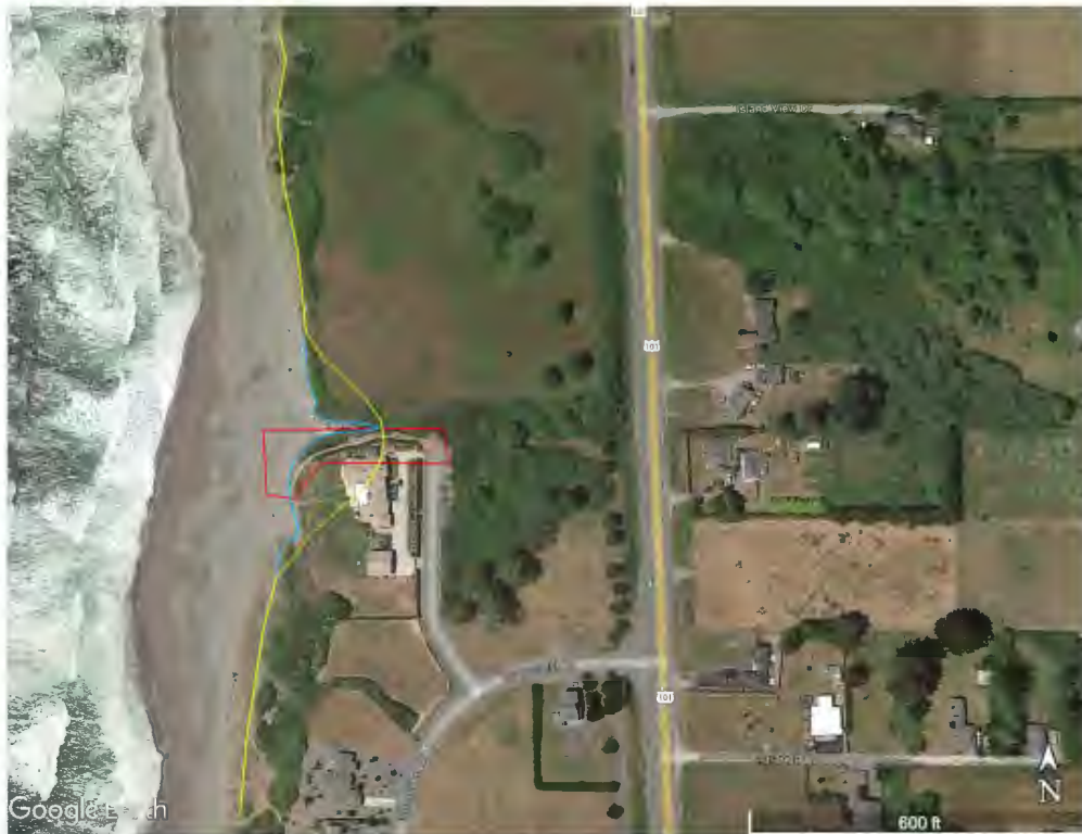
Figure 8: Modified Google Earth image showing estimated retreat of the access walkway located in the gully in 50 years. Red outline is project area, blue line is existing bluff edge, yellow line is 50-year retreat extent. Note that the blue and yellow lines overlap north and south of the project area.
