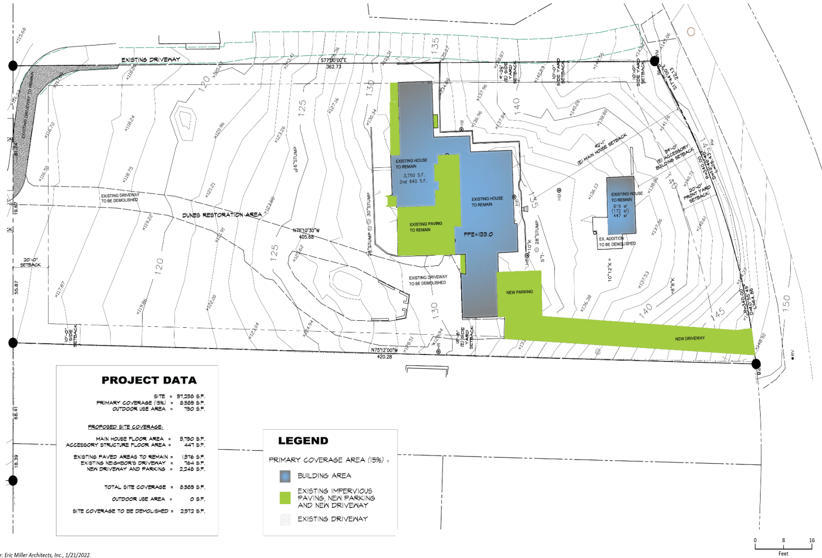
Figure 2-6 Project Site Plans: Existing Residence Site Plan
