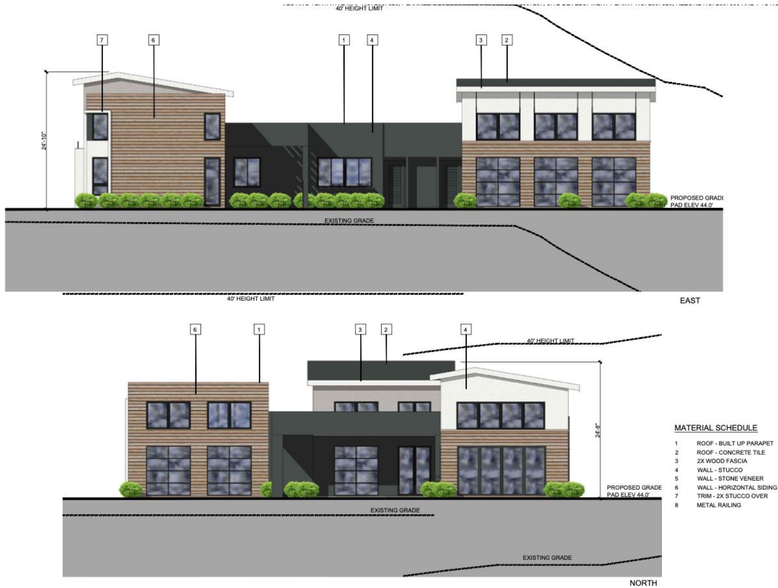
Figure 3-2h. Project Elevations – Rec/Leasing Building Elevation
