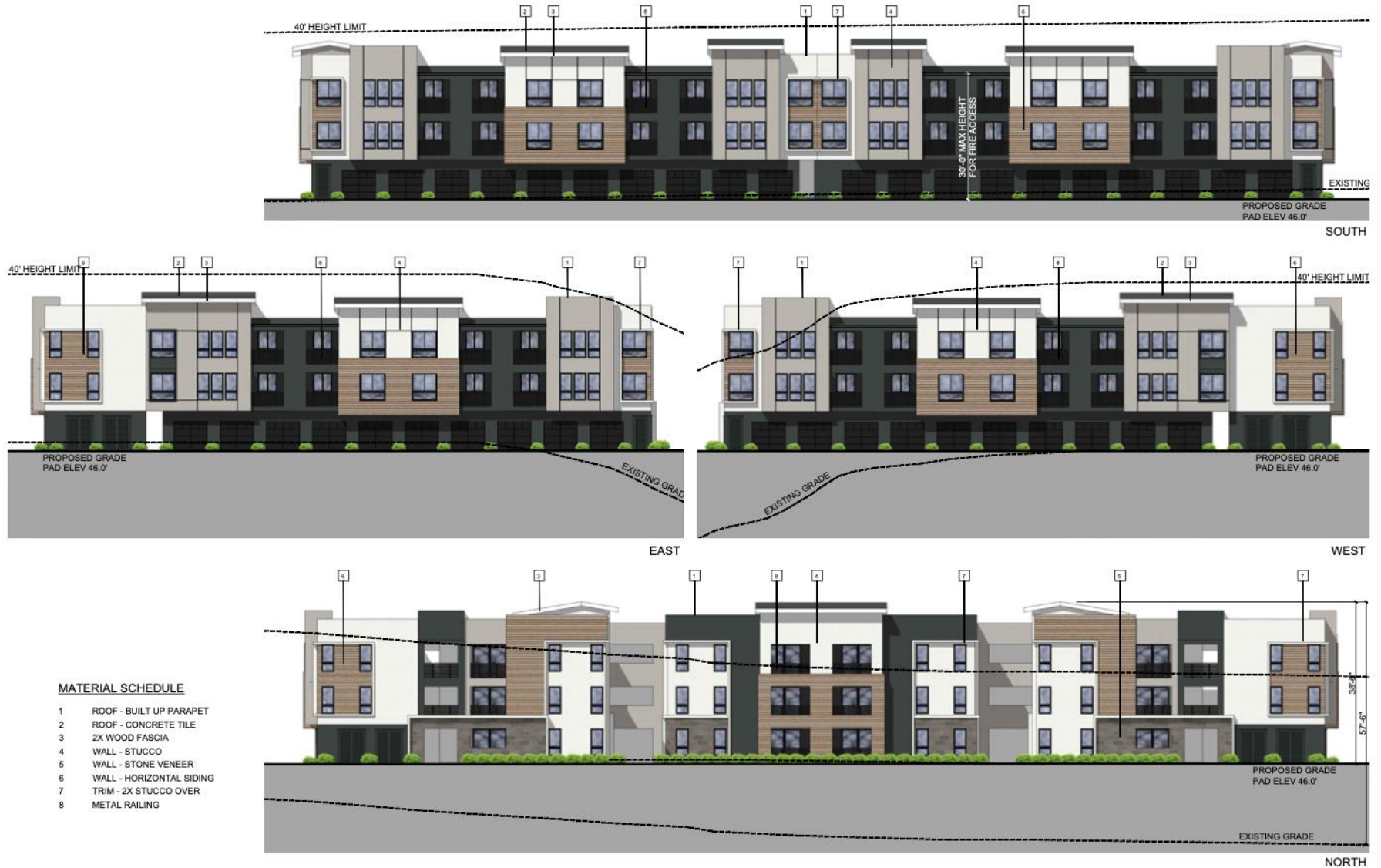
Figure 3-2e. Project Elevations – Building D Elevation
