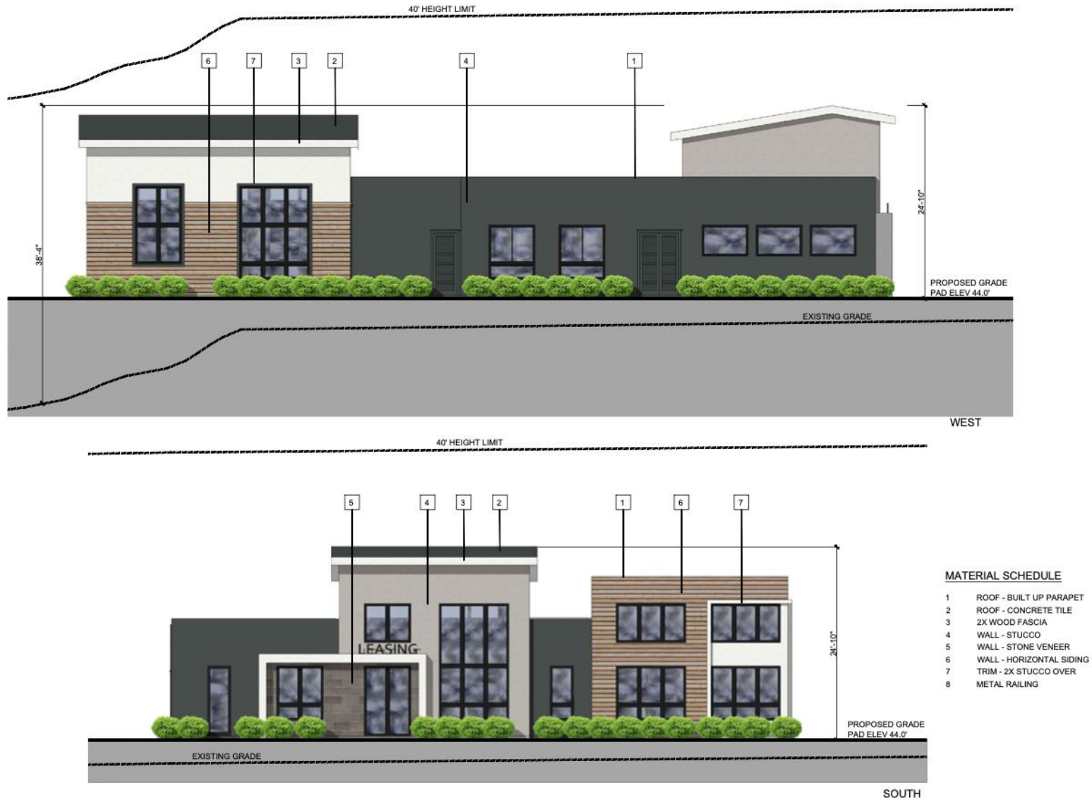
Figure 3-2g. Project Elevations – Rec/Leasing Building Elevation
