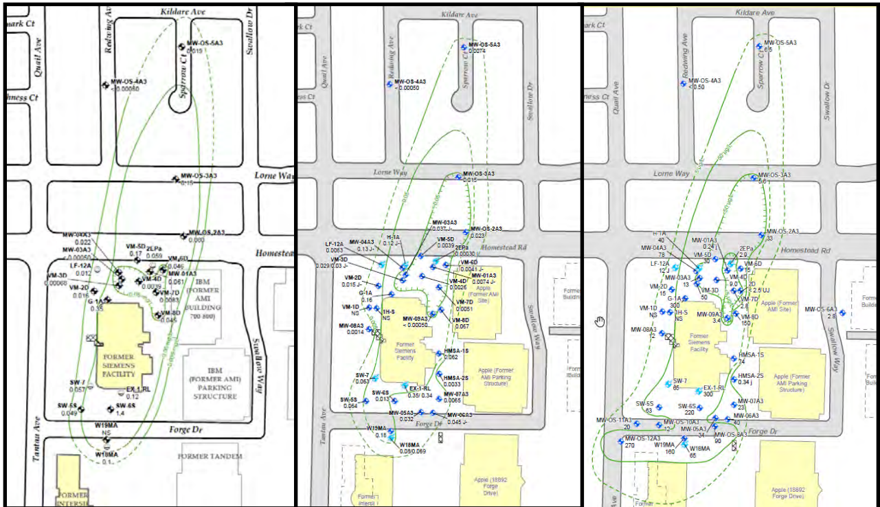
Figure C-2. TCE Plume in A3 Zone; 2015(mg/L), 2018(mg/L) and 2019(µg/L) (Left to Right) (AMEC Foster Wheeler and ERM, 2016; Wood and ERM, 2019 & 2020); isoconcentration images are in different units, however, the contours are equivalent (0.05 mg/L=50 µg/L).
