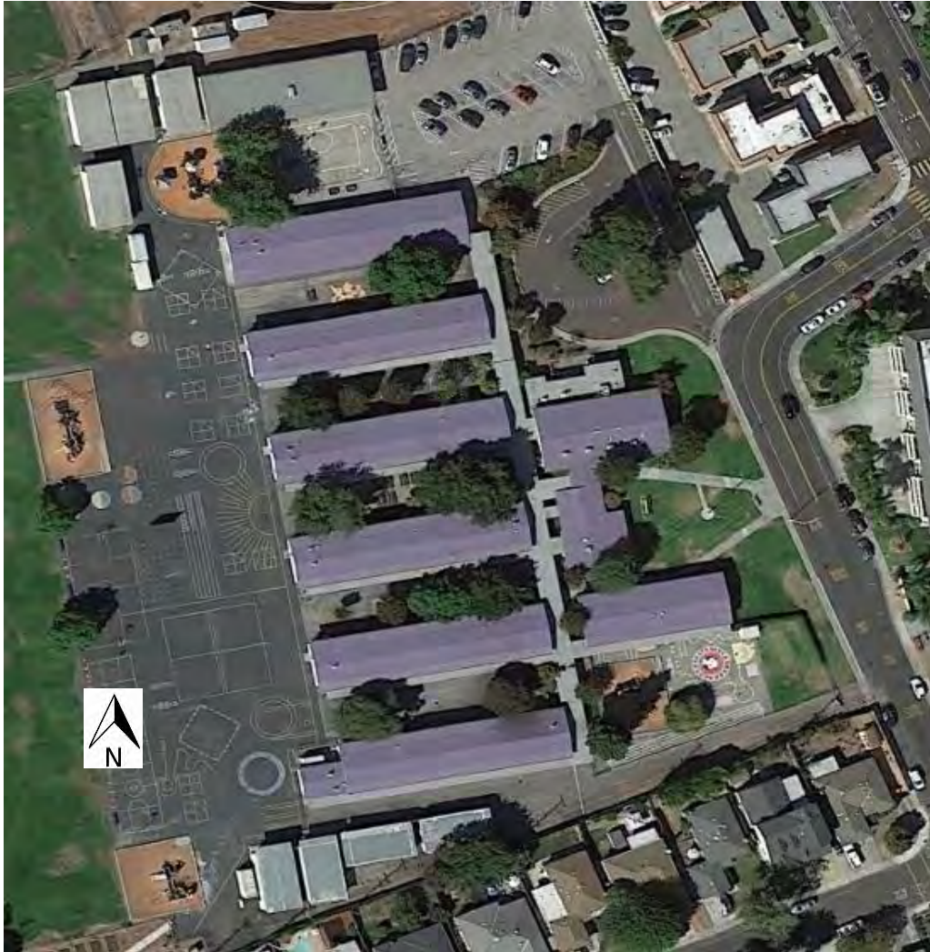
Figure 25. Typical "Finger-Plan" campus type. Briarwood Elementary School, Santa Clara. Built 1954-1956. GoogleEarth Pro. Accessed 5/18/2022. Image date 9/4/2020.
