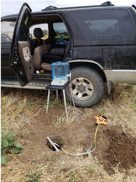
The Aardvark Permeameter was utilized in replacement of the Guelph Permeameter as recommended by Soil Moisture Equipment Corporation, due to the higher reliability, accuracy, and ease of use. The Aardvark Permeameter is the latest version of the Guelph Permeameter.
