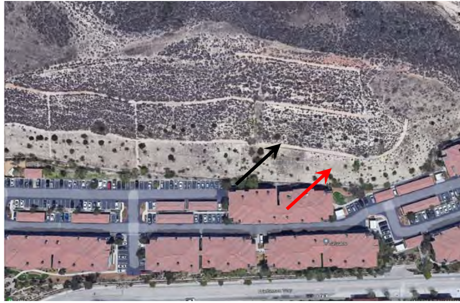
Photo 5 - Aerial View of a Portion of the Southern Boundary of the Project. Wildland fuels are present between the existing development to the south and the Project. The southern edge of the Project is located near the top of the manufactured slope identified by a black arrow. The owners to the south are maintaining 100 feet of fuel treatment (red arrow) between the Project and their buildings as can be seen above.
