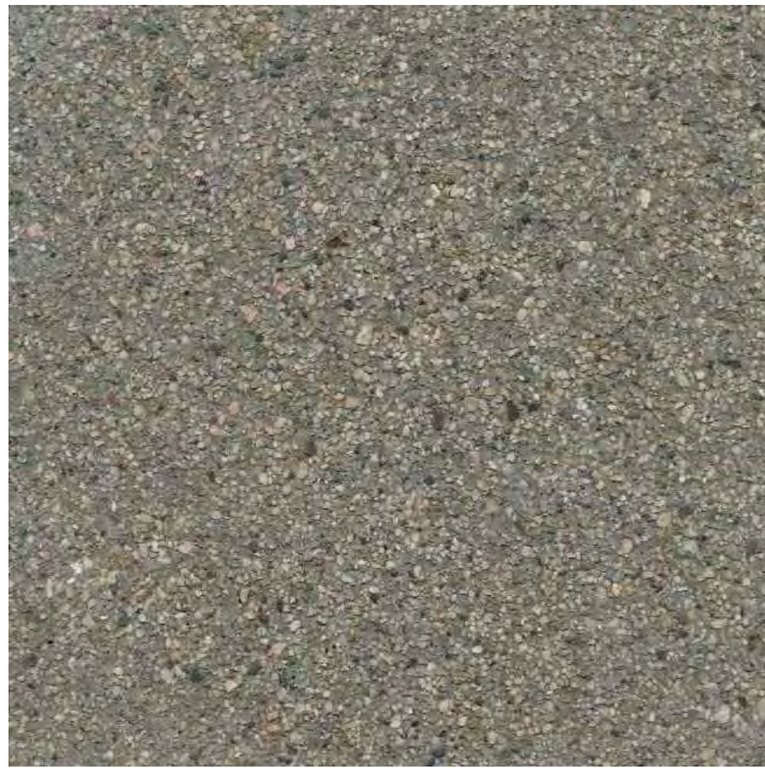
NATURAL COLOR CONCRETE W/ ACID ETCH OR TOPCAST FINISH AT BUILDING ENTRIES & EMPLOYEE PATIOS
