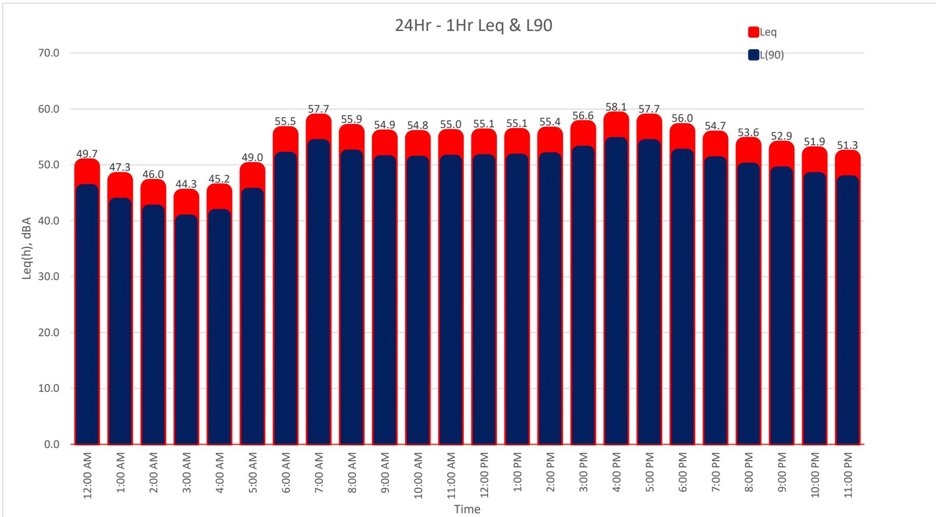
**24-Hour Continuous Noise Measurement Datasheet**
