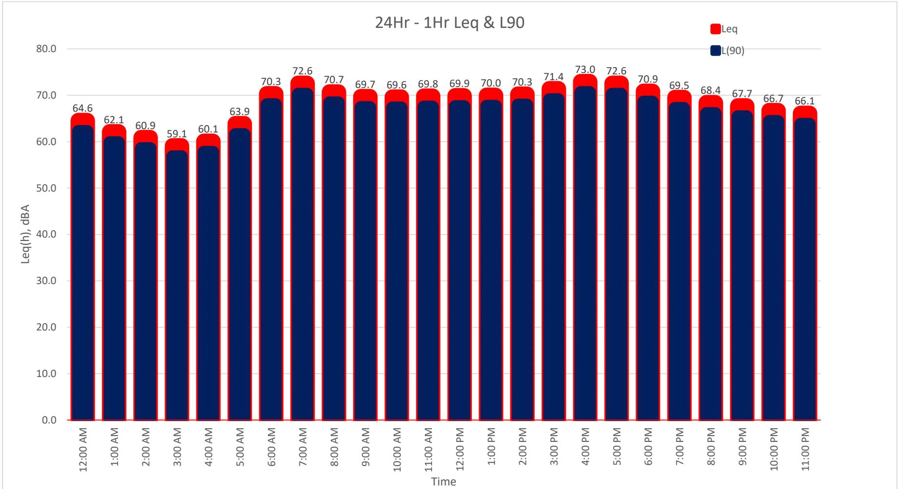
**24-Hour Continuous Noise Measurement Datasheet**
