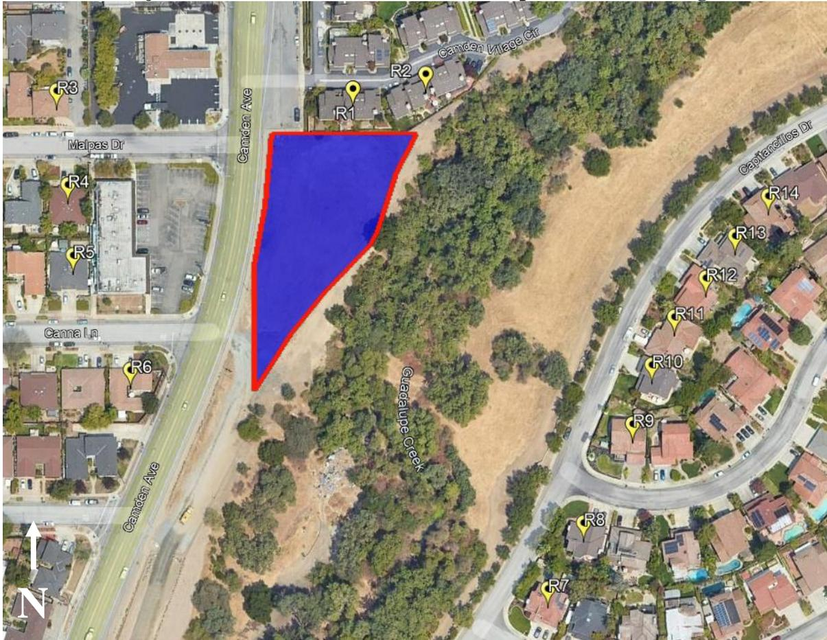
The construction noise levels were calculated to range from 75 to 86 dBA  $L_{eq}$  at 50 feet, using FHWA’s Roadway Construction Noise Model (RCNM), which assumes that all the equipment could be operated simultaneously. At the closest residence (R1) located about 100 feet to the north (along Camden Village Circle), hourly average noise levels are calculated to range from about 66 to 80 dBA  $L_{eq}$  (as shown in Table 6).
