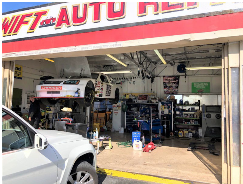
Photo 2. View of inside auto repair bay – two belowground hydraulic hoists, tool and chemical storage along back wall. Photograph taken March 16, 2021.
