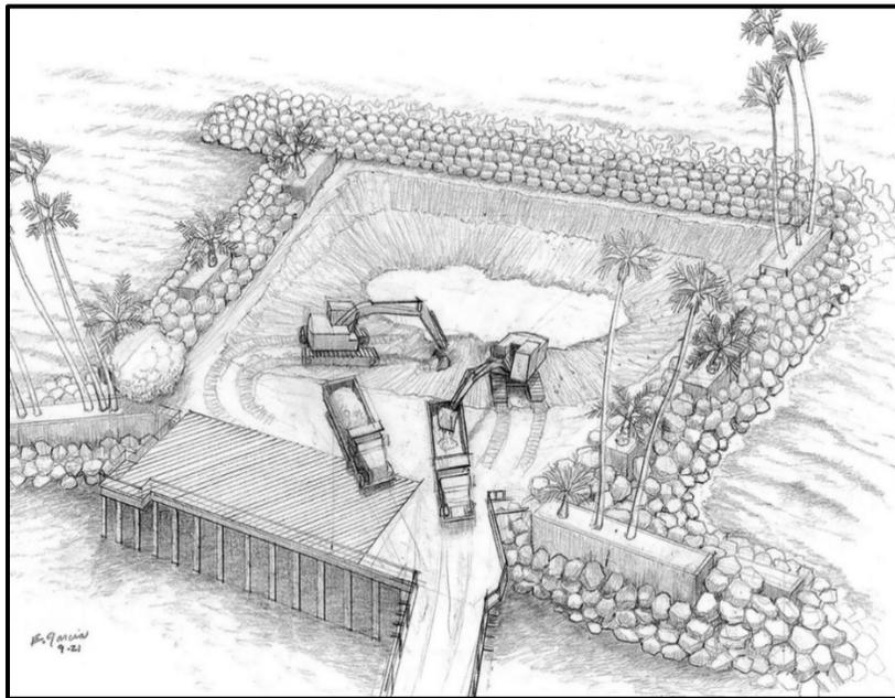
**Figure 11. Illustration of Island Backfill and Compaction**
