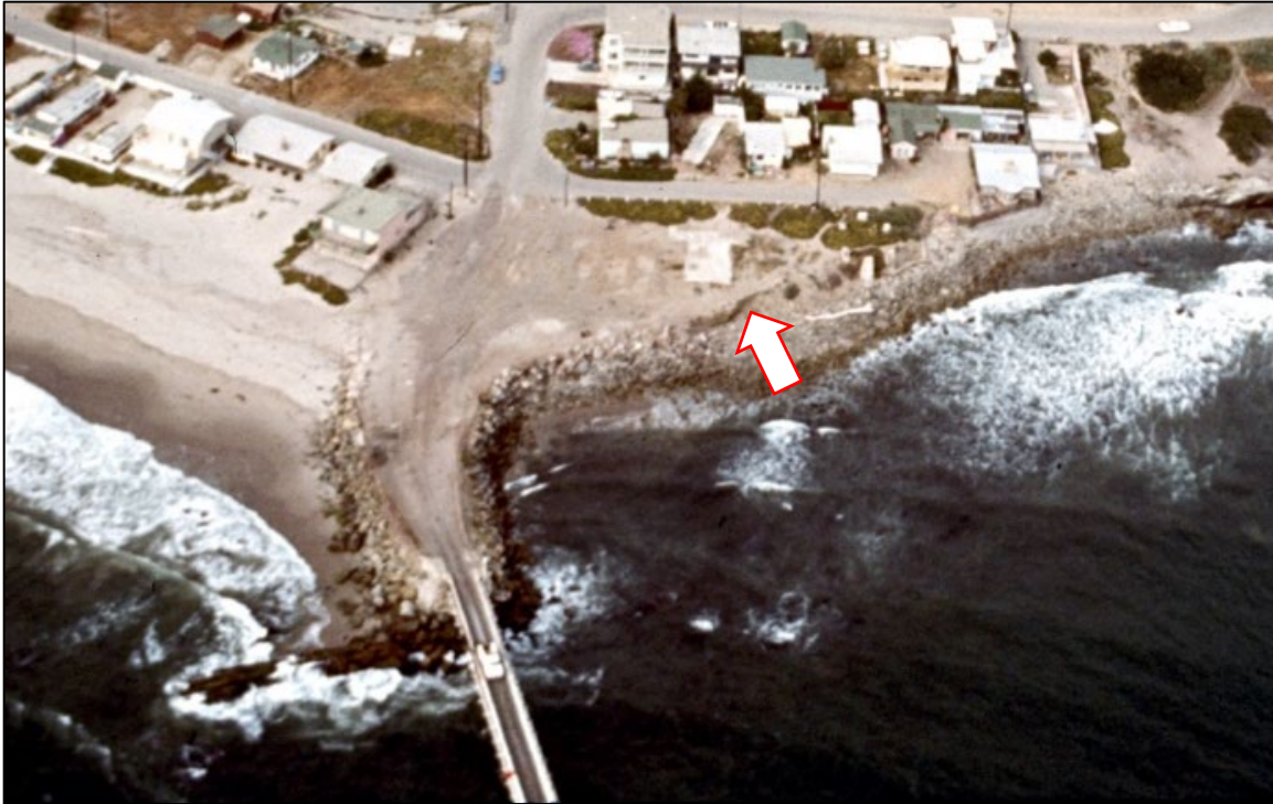
Figure 9. SCC site in 1972. The downcoast or eastern side of the parcel shows a rocky beach but no riprap and a scarp that has been eroded into the low unarmored bluff (arrow) (California Coastal Records Project - Kenneth and Gabrielle Adelman).
