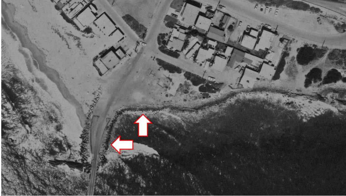
Figure 8. State Coastal Conservancy parcel in 1971 with riprap armoring the right side of the abutment and continuing downcoast in an arc along a portion of the shoreline (arrows).
