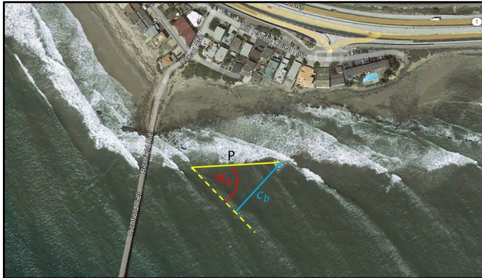
Figure 3-6. Definition Sketch of Peel Angle, Wave Celerity, and Peel Rate
