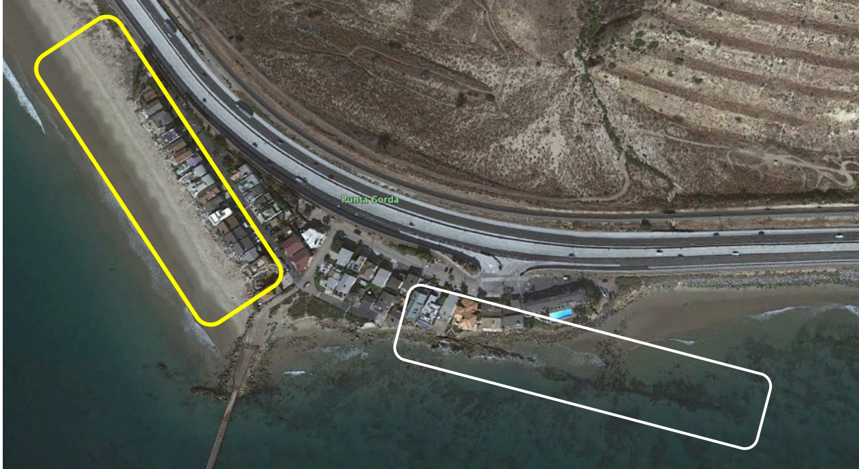
Figure 20. Beach upcoast of Punta Gorda showing encroachment of homes on the shoreline that reduced beach width (outlined in yellow), and downcoast rocky shoreline. Note Pico Formation bedrock outcropping along the back beach extending into the subtidal (outlined in white)(Google Earth August 2019).
