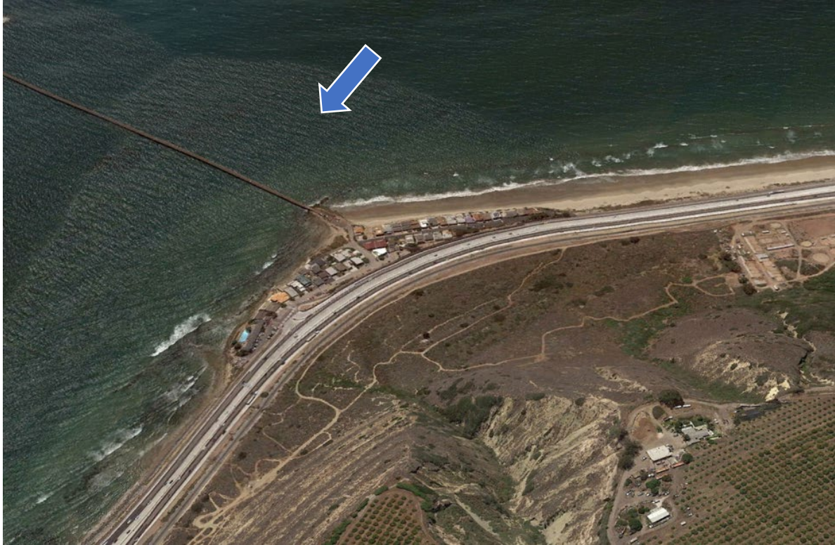
Figure 25. May 2015 Google Earth image showing wave fronts approaching from the WNW (from approximately 280°) and striking the upcoast sandy beach before reaching the causeway.
