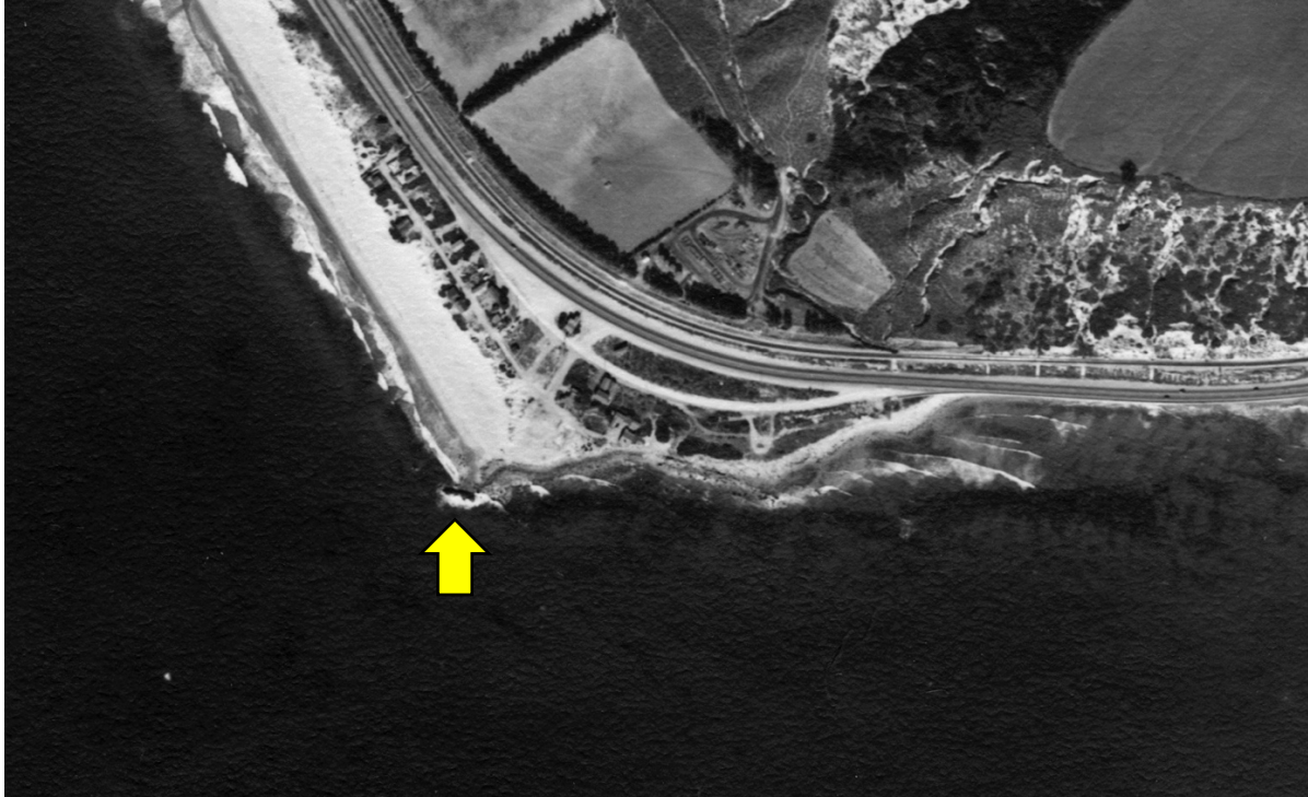
Figure 19. Punta Gorda in November 1945 showing Pico Formation bedrock trapping sand and forming the point.
