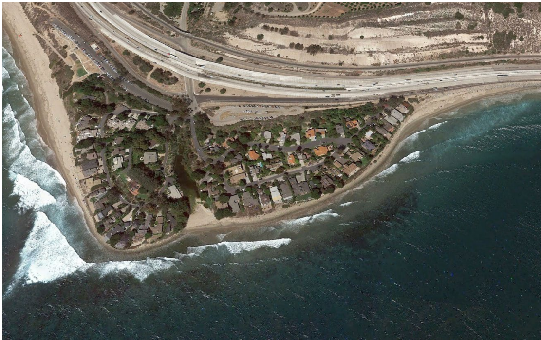
Figure 16. Rincon Point in August 2014 showing wave refraction around point and narrow beach immediately downcoast.
