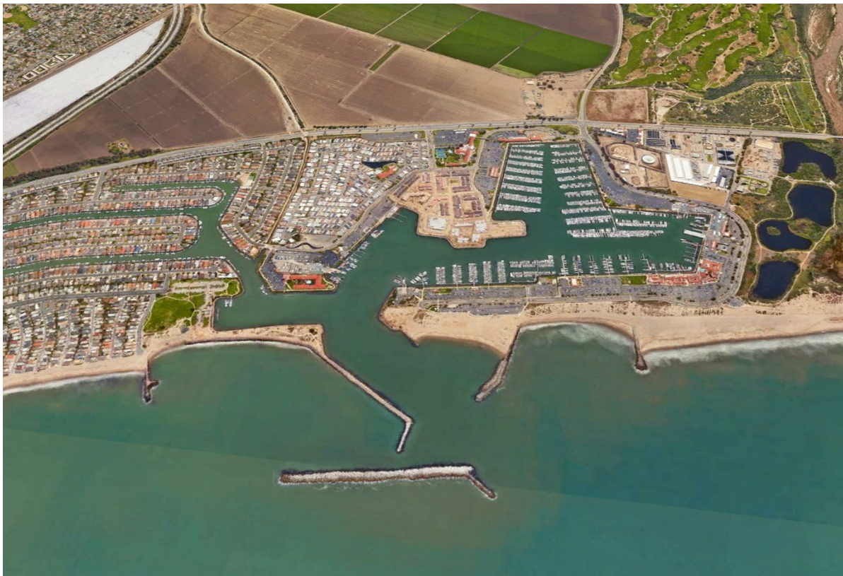
Figure 6. Ventura Marina, 10 miles east of Punta Gorda, where an average of about 600,000 \text{ yds}^3 is dredged annually. Littoral drift of sand moves from left to right.
