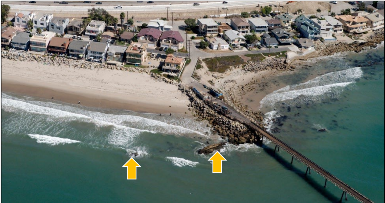
Figure 8. Nearshore bedrock outcrops forming Punta Gorda adjacent to left side of abutment (2013 photo from California Coastal Records Project, Kenneth and Gabrielle Adelman).
