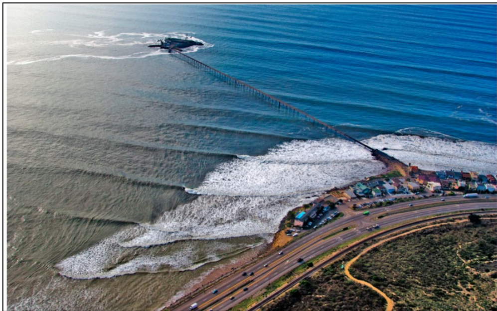
Figure 32. December 21, 2006, aerial photograph of swell approaching Mussel Shoals and passing unchanged through the causeway during what has been called the largest swell in a decade (© Anthony Ghiglia).
