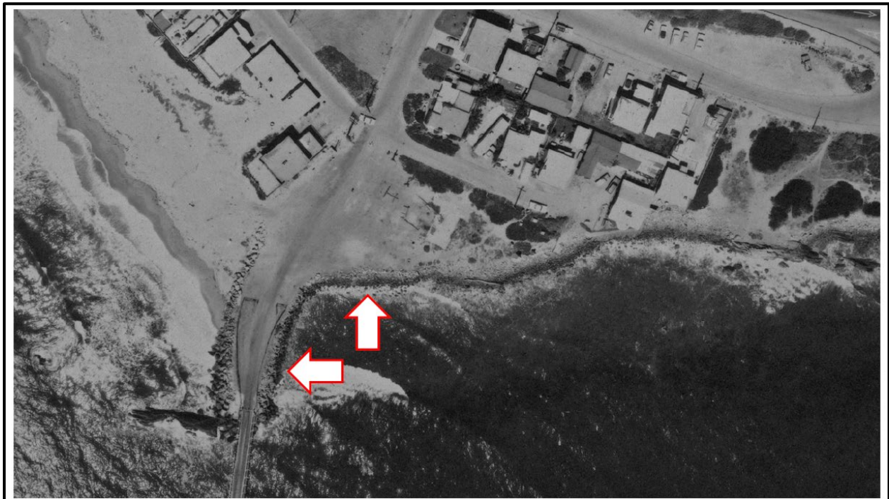
Figure 4.6-4. Riprap Present Along SCC Parcel Shoreline (Photo From 1971, Riprap Placed Before This Time)
