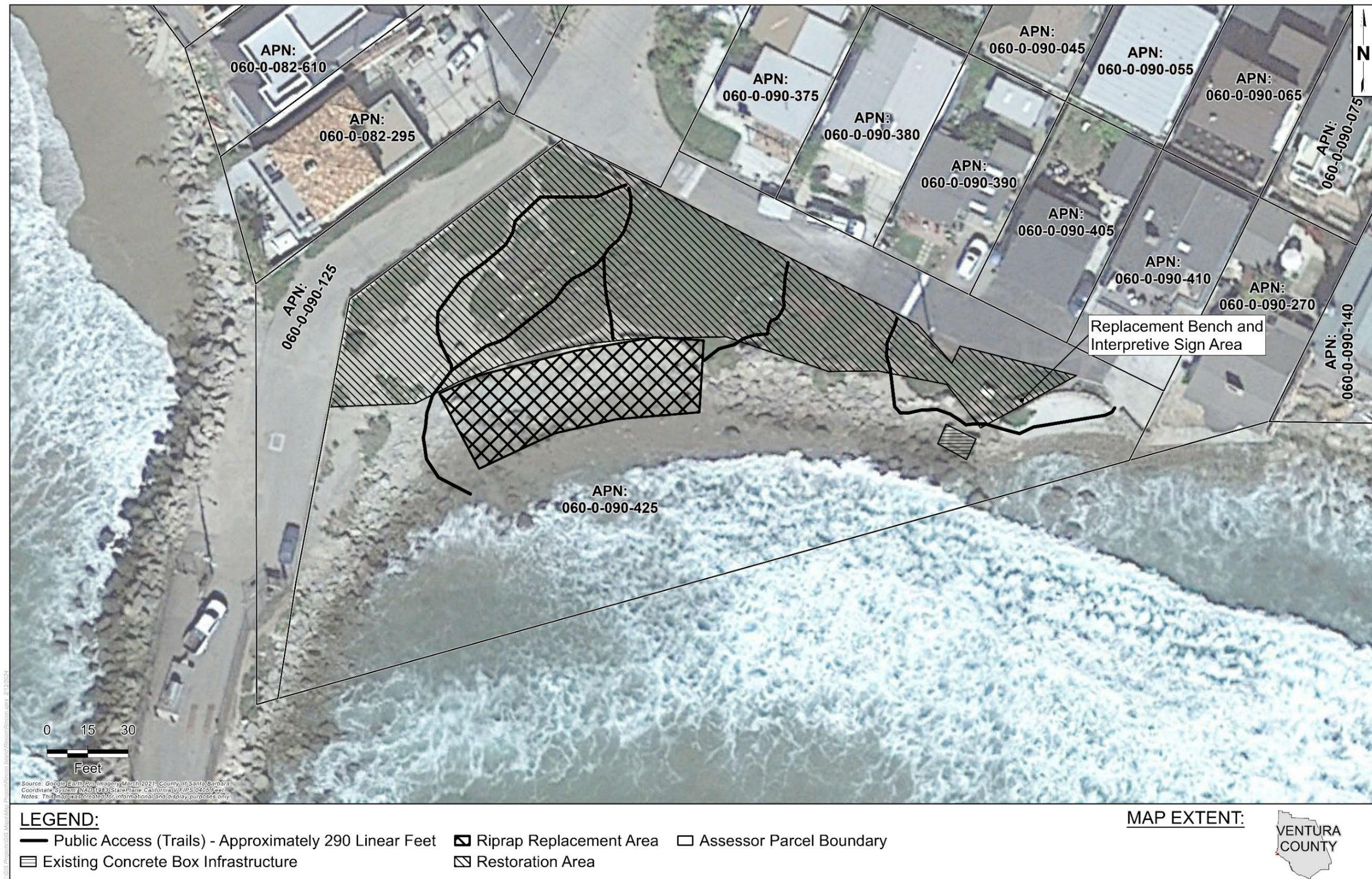
Figure 2-24. SCC Parcel – Option 3: Native Revegetation, Access Improvements, and Installation of Riprap Along Parcel Frontage
