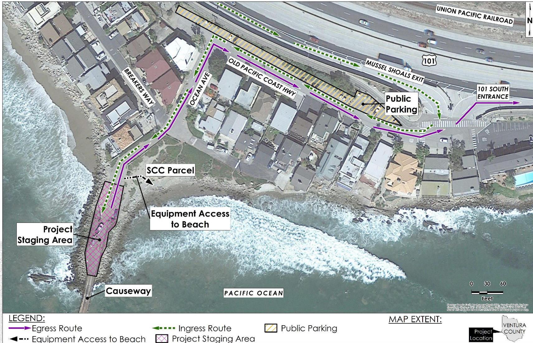
Figure 2-28. Access and Staging – Rincon Island Causeway and SCC Parcel Areas
