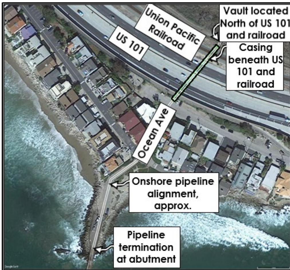
Figure 2-25. Onshore Pipeline Connections
