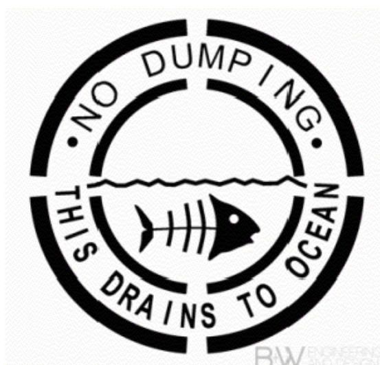
CATCH BASIN STENCILING DETAIL NTS
