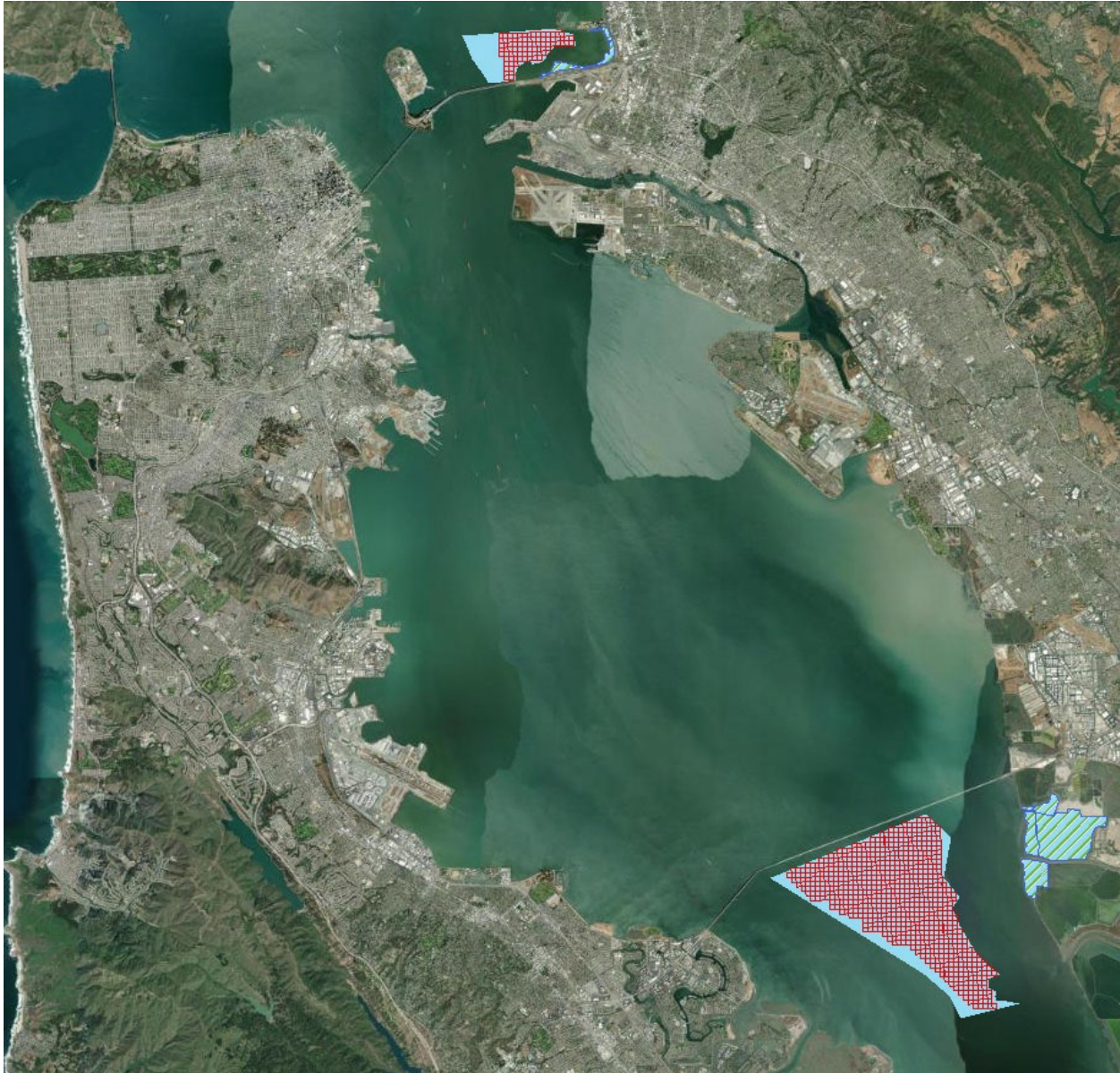
Figure 3-2. Strategic placement sites narrowed down from twelve to two: Emeryville (top) and Eden Landing (bottom). Site map includes both placement footprint (red grid) and target marsh for restoration (aqua hatch).
