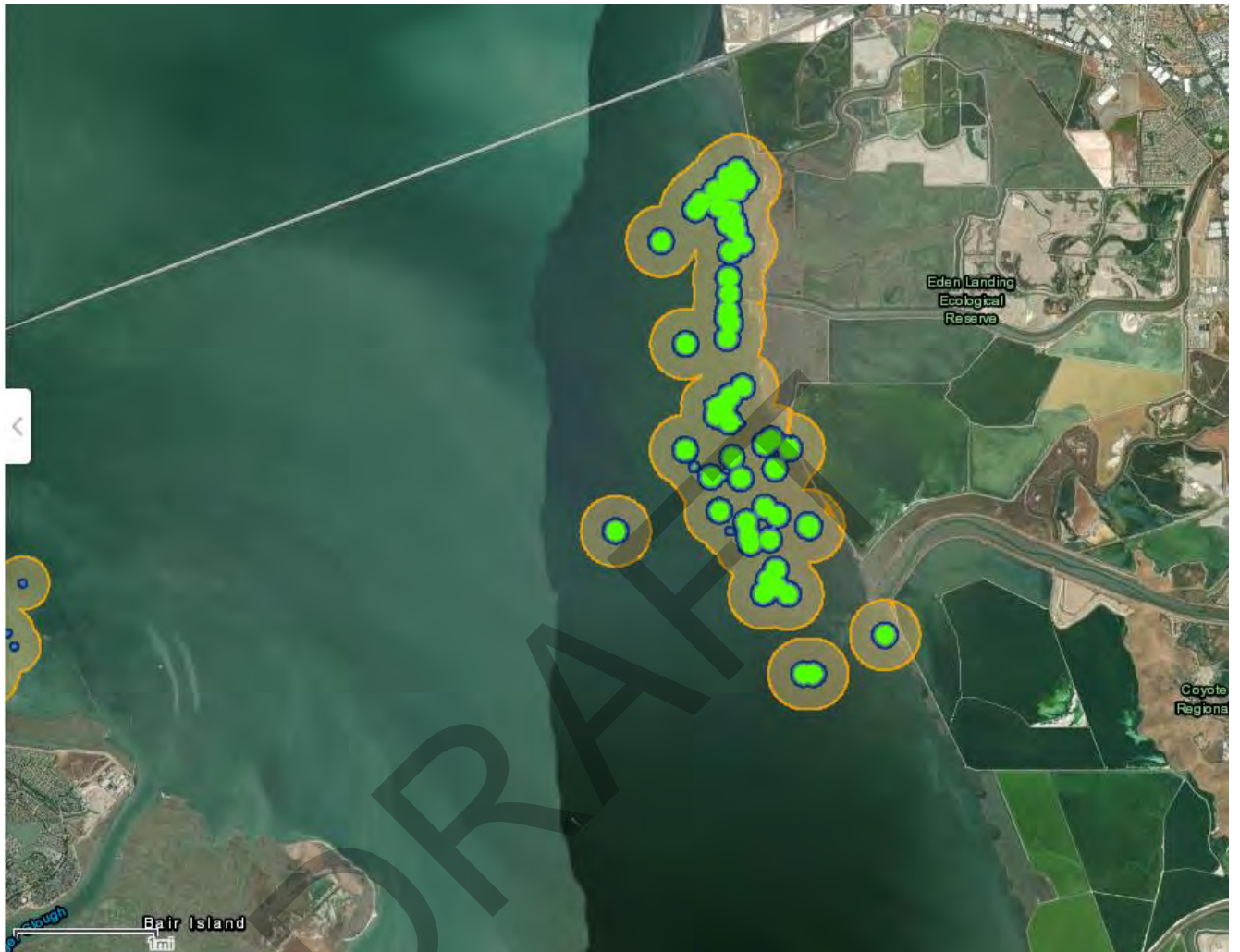
Figure 3. Eelgrass mapped near Eden Landing. Includes data from surveys conducted in 2003, 2009, 2013, and 2019. The orange border indicates the 250 m turbidity buffer from NMFS (2011). A comparison with Figure 1 indicates no encroachment of the dredge disposal site into the turbidity buffer. Source: San Francisco Bay Eelgrass Impact Assessment Tool | CNRA GIS Open Data (ca.gov)
