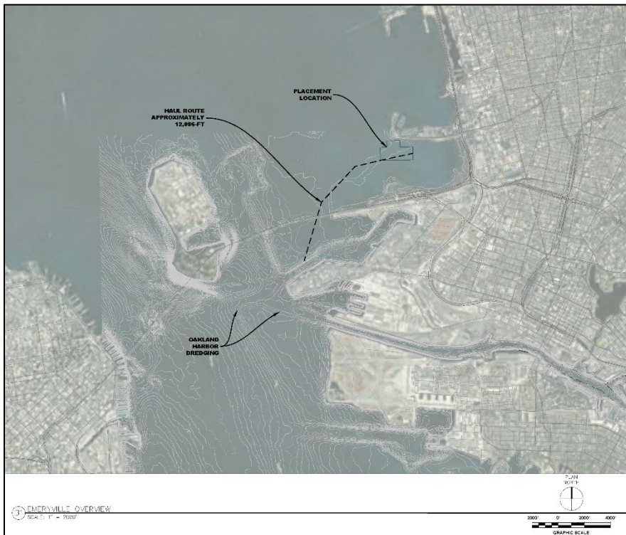
Figure 3-6. Haul Routes from Oakland Harbor to the nearshore Emeryville Crescent placement site.
