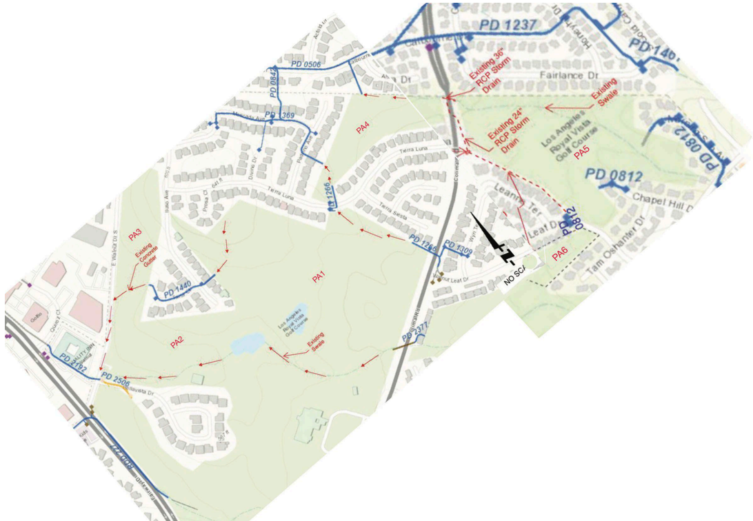
FIGURE 2 – Existing Drainage On The Project Site Source: DEIR Figures 4.10-1
