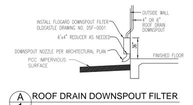
**A** ROOF DRAIN DOWNSPOUT FILTER
