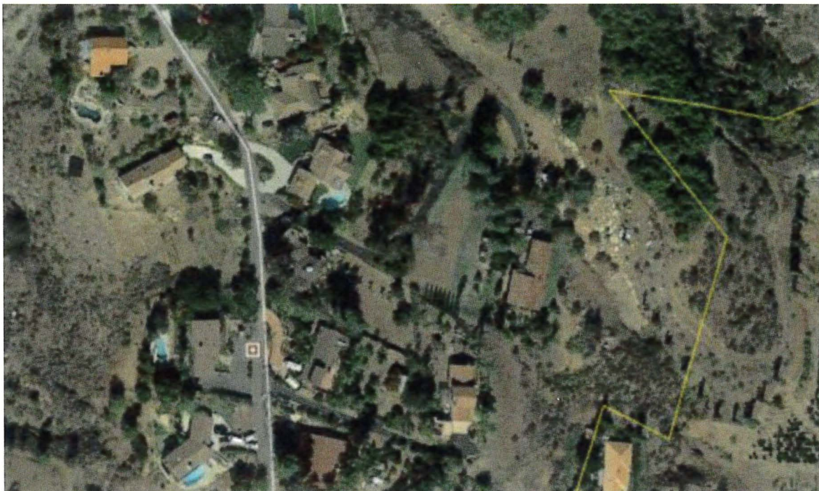
Figure 4. Example of moderate density development. Homes are located on larger properties and include varying levels of ignition resistance and landscape / fuel modification provision and maintenance. This type of development results in a higher wildland exposure level for all homes and does not provide the same buffers from wildfire encroaching onto the site, or starting at a structure and moving into the wildlands as a higher density project.
