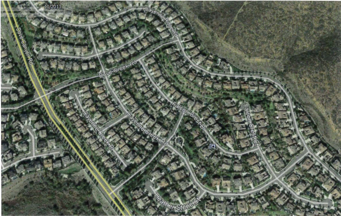
Figure 3. Example higher density development that is ignition resistant and excludes readily ignitable vegetative fuels throughout and provides a perimeter fuel modification zone. This type of new development requires fewer fire resources to defend and can minimize the likelihood of on-site fires spreading off-site.
