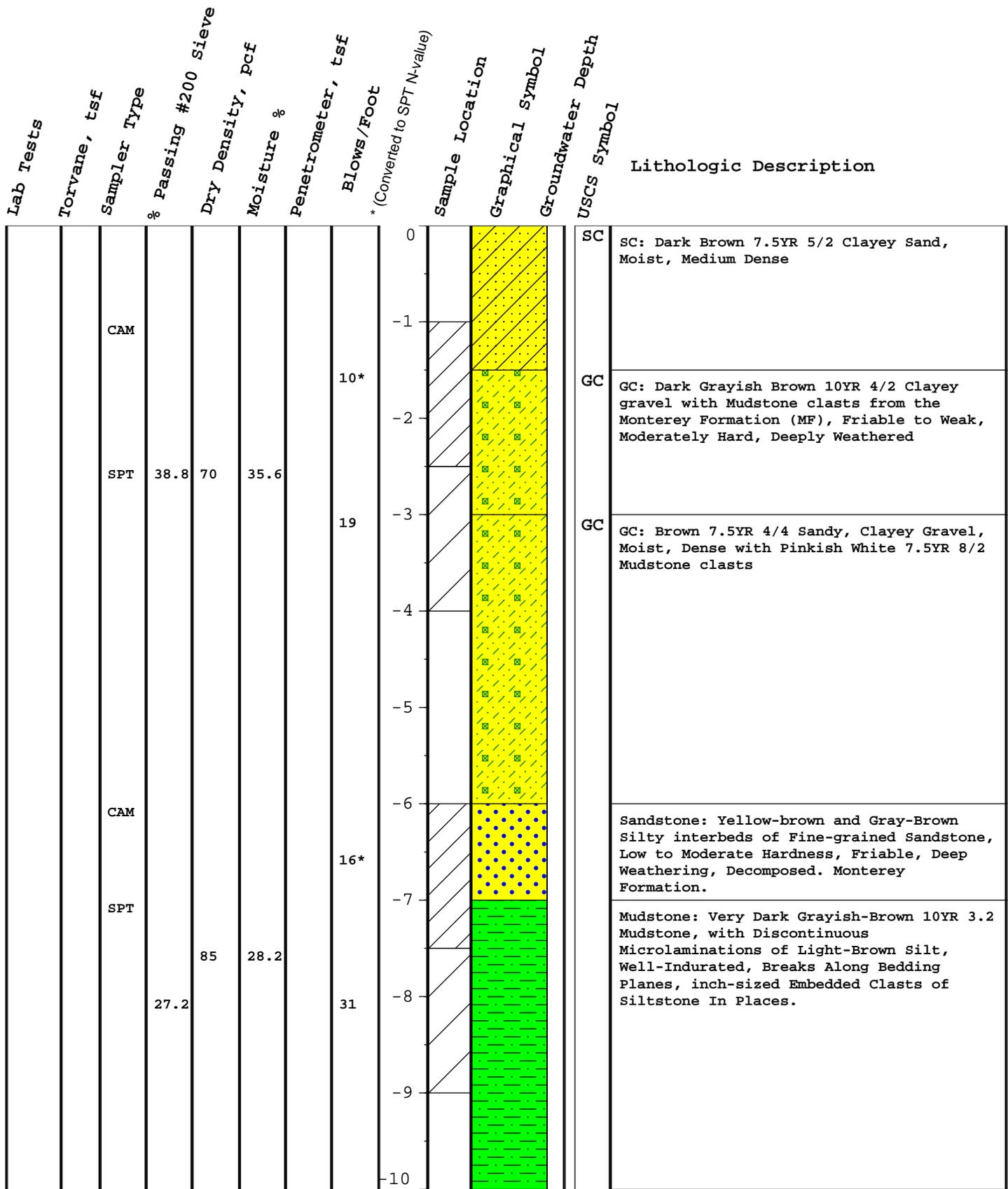
\*Sampling was performed by Denovo Drilling using a hydraulic portable drill rig equipped with solid flight augers.
