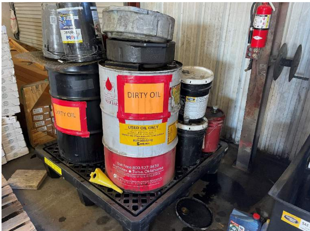
Photo 14: Used oil drums with staining on pavement around secondary containment.
