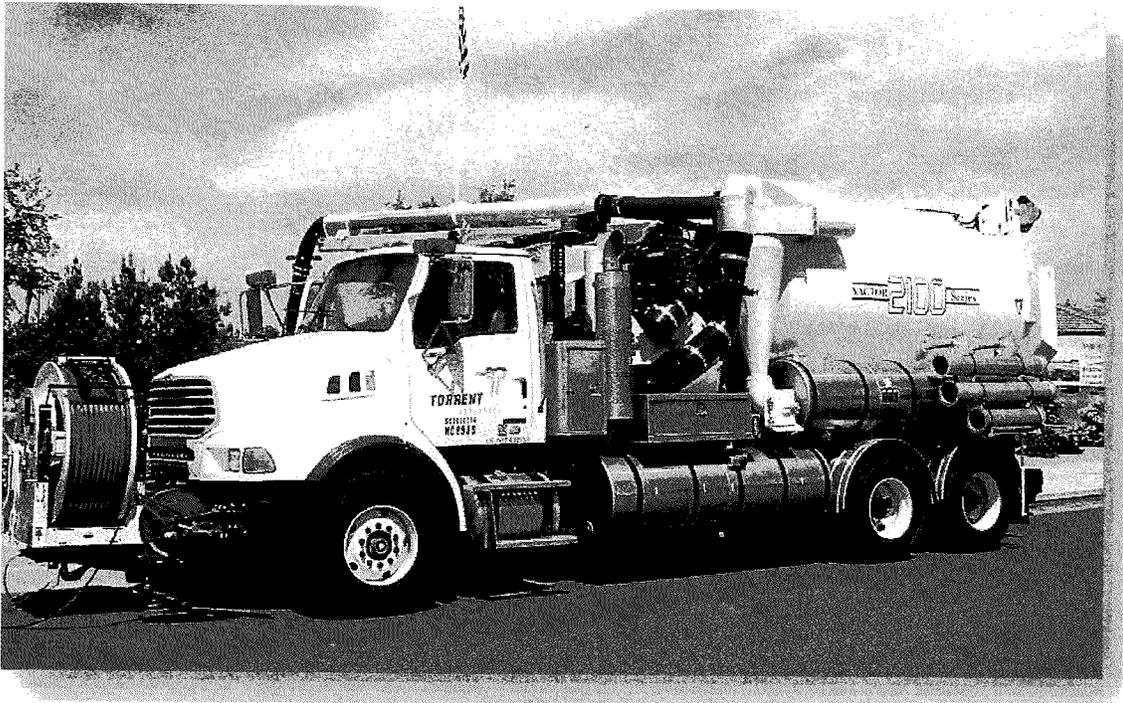
*Typical hydro-vacuum truck used for drywell maintenance*
