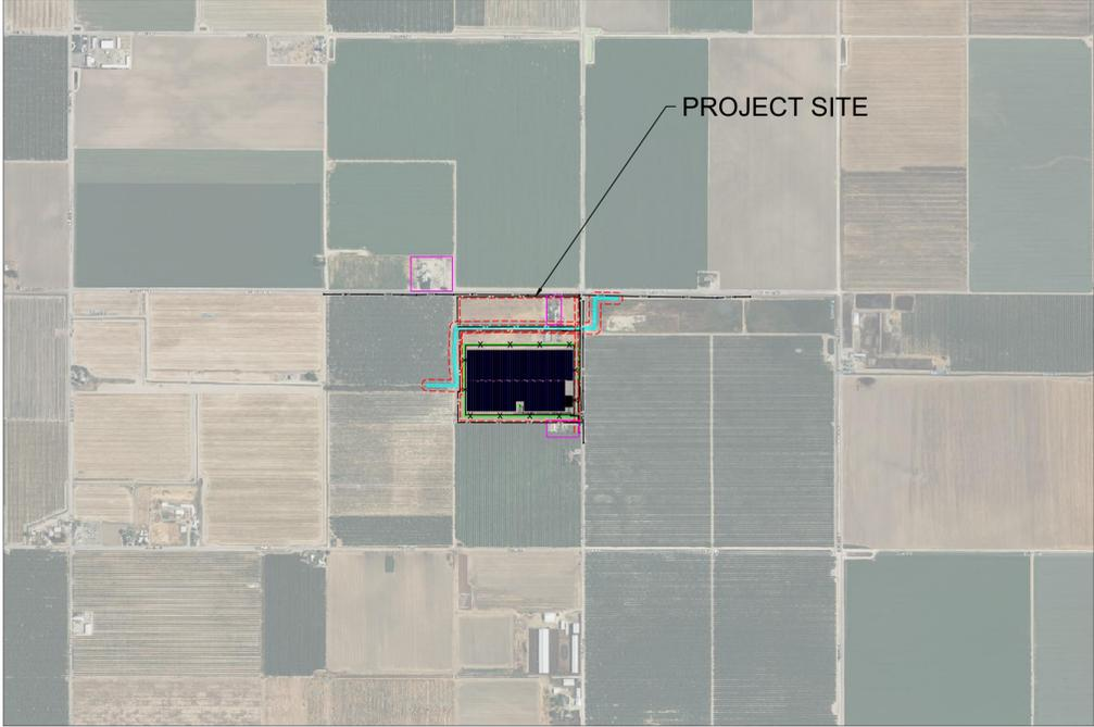
DEVELOP NEW SOLAR PHOTOVOLTAIC ELECTRICAL GENERATING FACILITIES ON APPROXIMATELY 18.35 ACRES OF LAND. THE SOLAR POWER PLANT WILL BE A SINGLE AXIS TRACKER SYSTEM. THE ENTIRE SITE WILL HAVE MINIMAL EARTHWORK DISTURBANCE AND GRADING OPERATIONS WILL OCCUR MAINLY FOR INSTALLATION OF ACCESS ROADS AND EQUIPMENT PADS.
