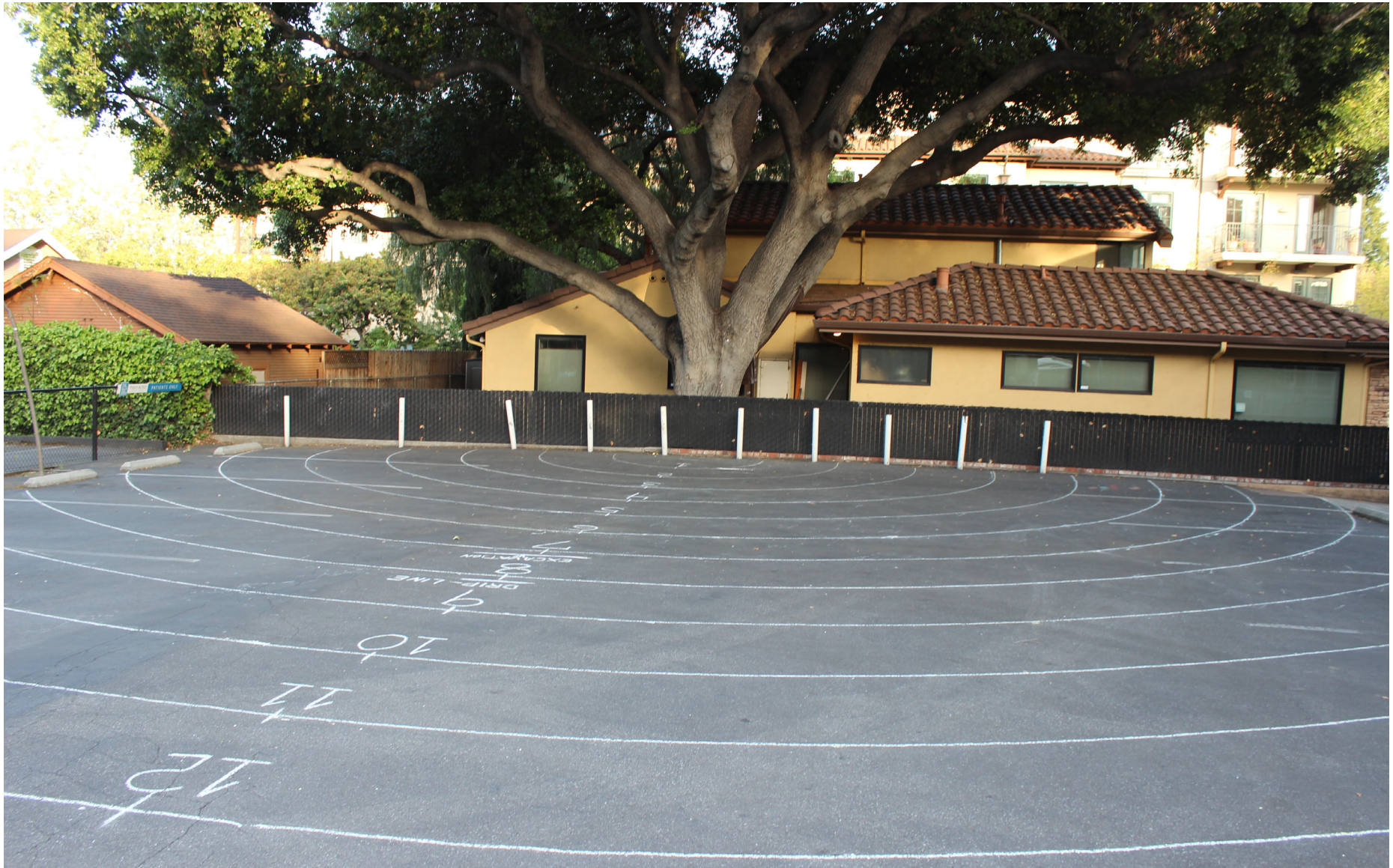
These chalk lines represent the locations of half circle scans. Scan #8 represents the edge of the canopy drip-line. Scan #7 represents the edge of the proposed excavation for the below ground garage about 30 feet away from the Oak tree.
