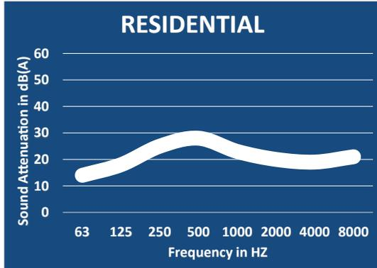
Nett Technologies' Residential Grade Silencers are designed to achieve maximum performance with the least amount of backpressure. The silencers are Reactive Silencers and are typically used for reciprocating or positive displacement engines where noise level regulations are medium-low.
