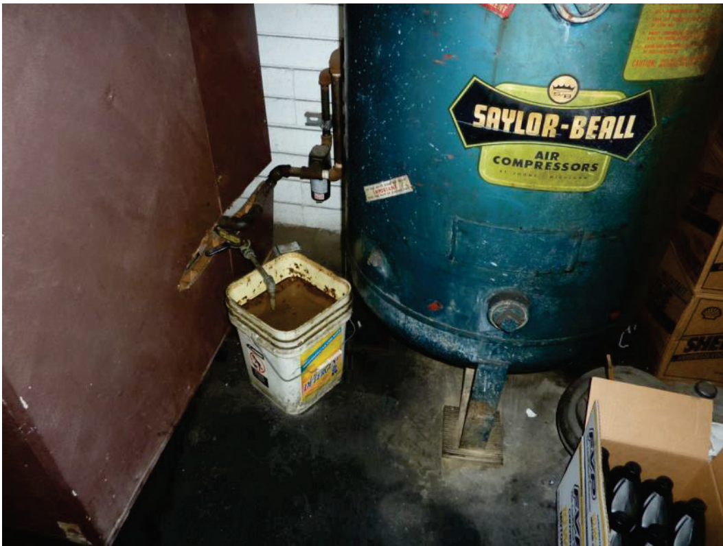
F-12. Air compressor and pail of oily condensate at Rusty's Automotive, 11522 Alondra (7/10/2014).
