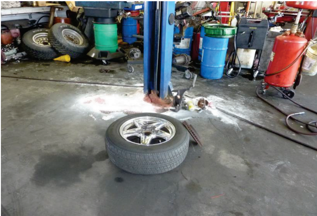
F-6. Oil sorb soaking up leaking hydraulic oil at Rusty's Automotive, 11522 Alondra (7/10/2014).
