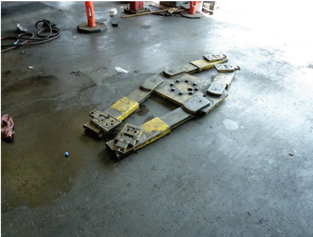
F-4. Typical in-ground hydraulic vehicle lift at Rusty's Automotive, 11522 Alondra (7/10/2014).
