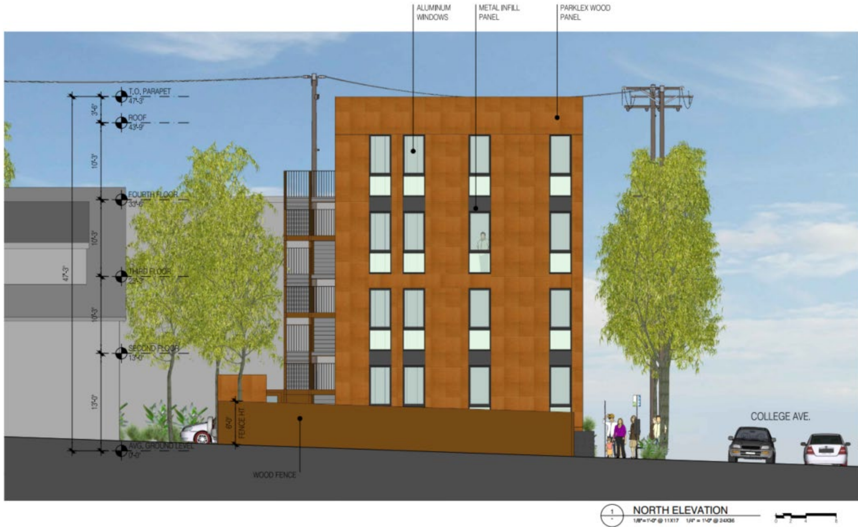
Figure 7. North View Elevations of the Building
