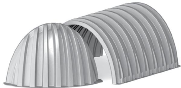
With all StormTech chambers, one chamber type is used for the start, middle and end of rows. Rows are formed by overlapping the upper joint corrugation of the next chamber over the lower joint corrugation of the previous chamber (**Figure 6**).
