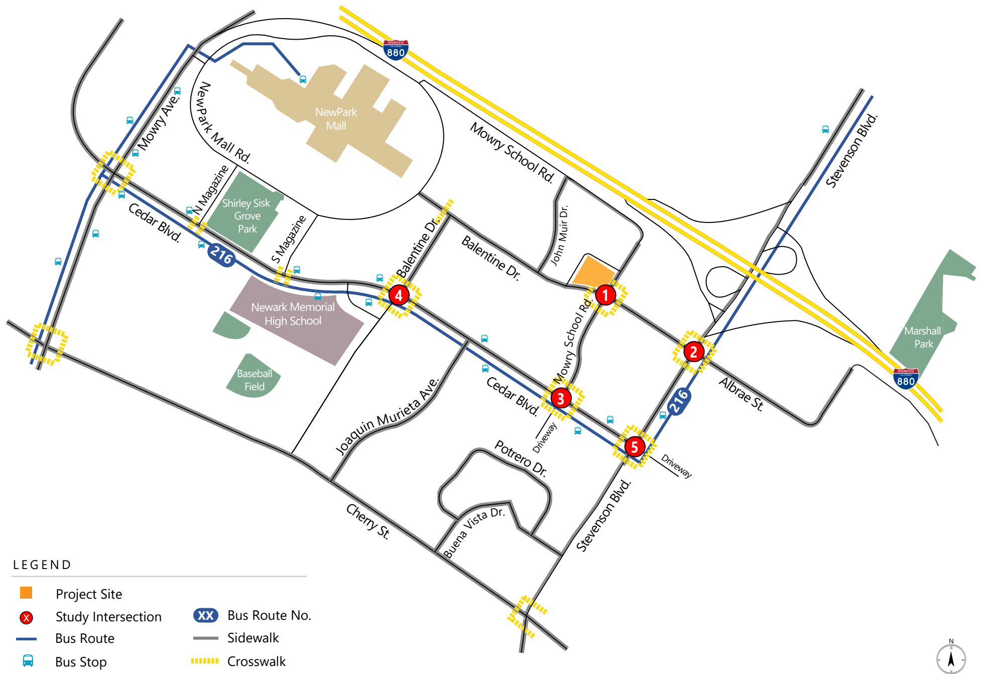
Figure 3: Existing Pedestrian and Transit Facilities
